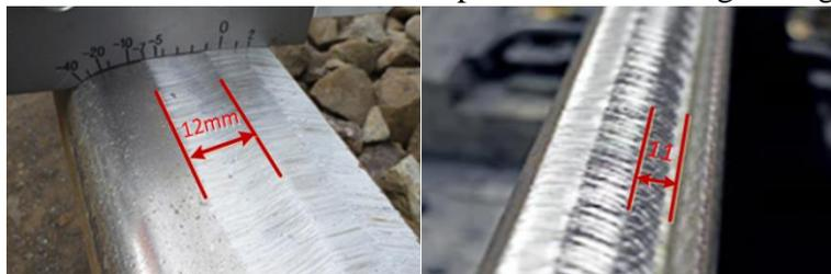
Fig.3 The lateral width specification of a grinded rail surface (unit: mm)
