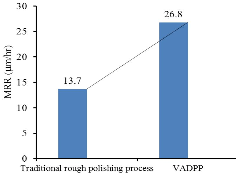
Fig. 4 MRRs of traditional rough polishing and the VADPP for the C-face of 4H-SiC wafer.
