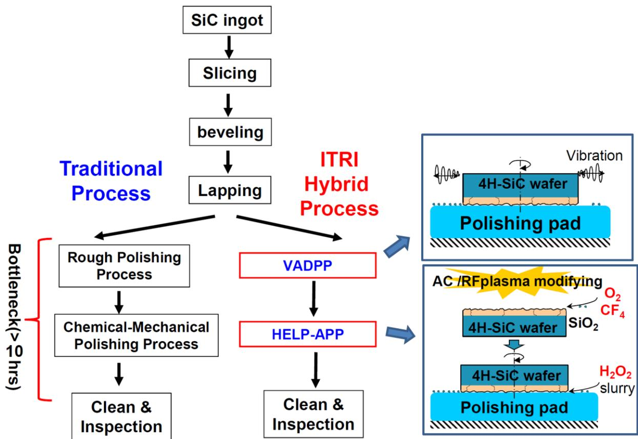
Fig. 1 Flowcharts of the ITRI innovation hybrid machining process and traditional machining process for the surface polishing of SiC wafer
