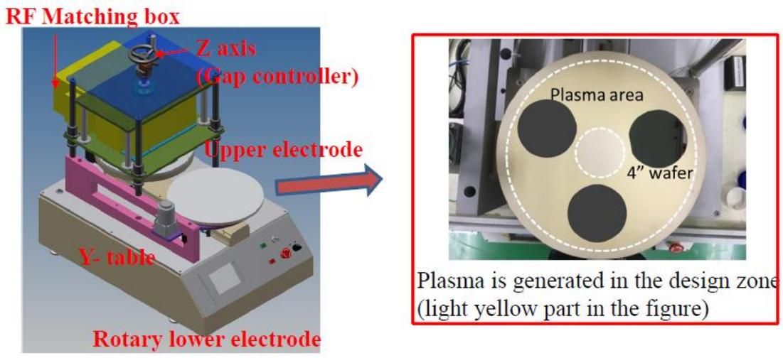
Fig. 3 Schematic of the HELP-APP module
