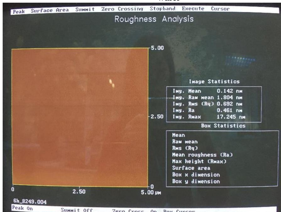
Fig. 6 Roughness analysis of the finished SiC wafer surface measured by AFM
