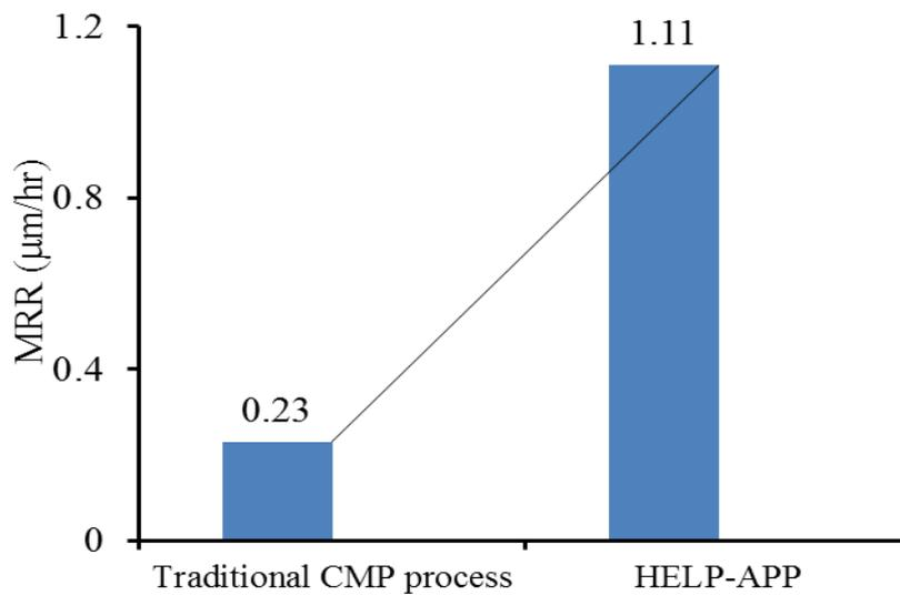
Fig. 5 MRRs of traditional CMP process and HELP-APP for the C-face of the SiC wafer
