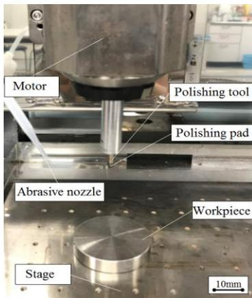
**Fig. 3** Photograph of experimental setup
