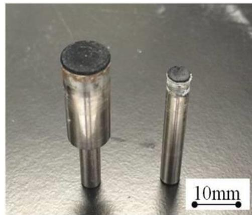
**Fig.4** Photograph of scan polishing tool (left:  $\phi 10$  mm, right:  $\phi 5$  mm)
