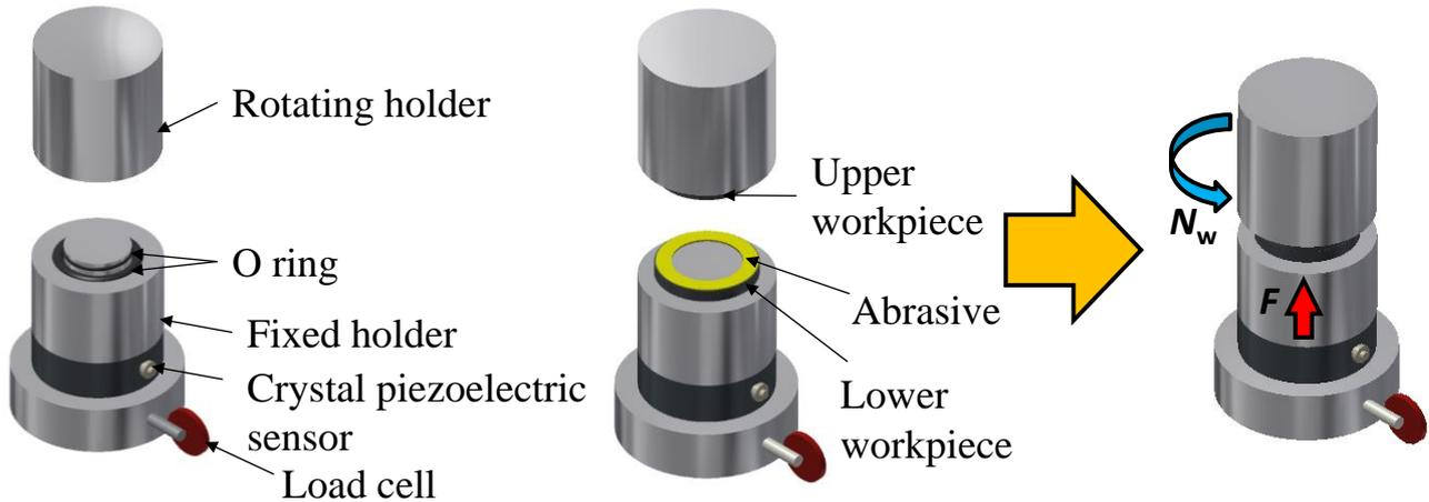
Fig.3 The schematic and steps of concentric mutual lapping
