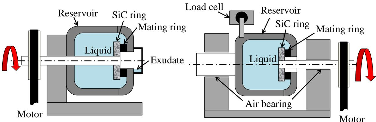
Fig.4 Exudate measurement testing machine
