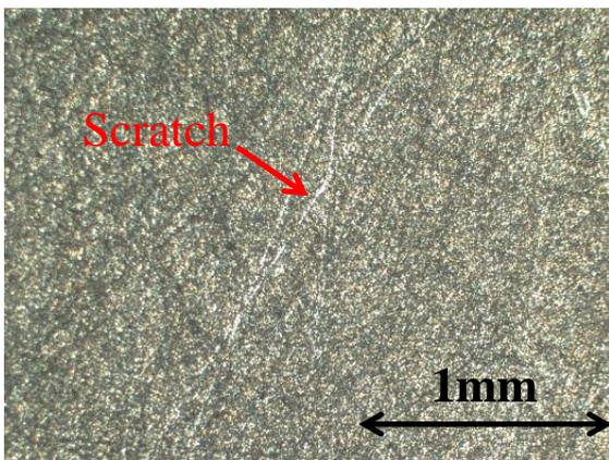
Fig.1 Conventional lapping surface
