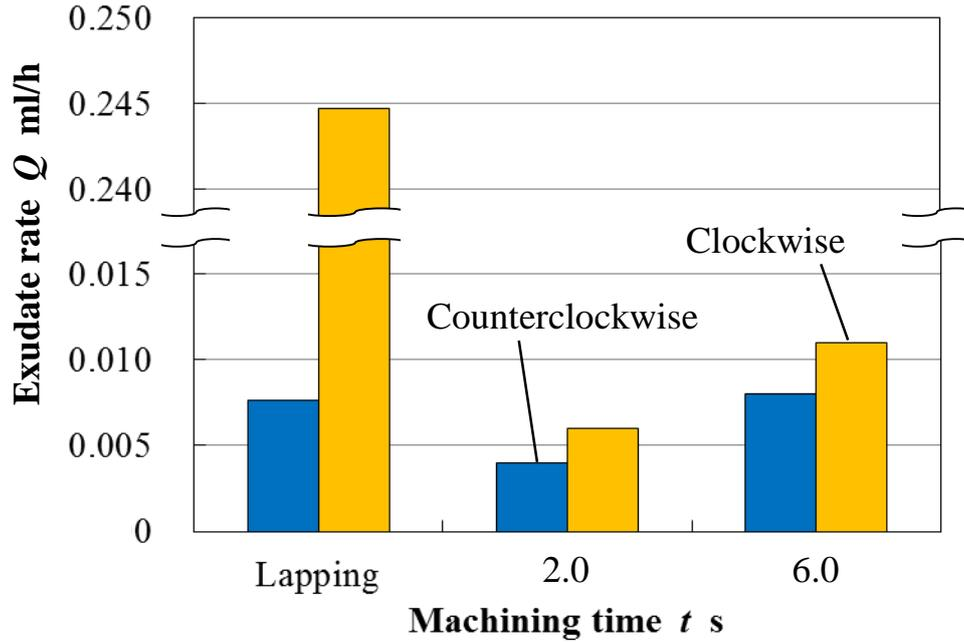
Fig.7 Relationship between machining time and exudate rate
