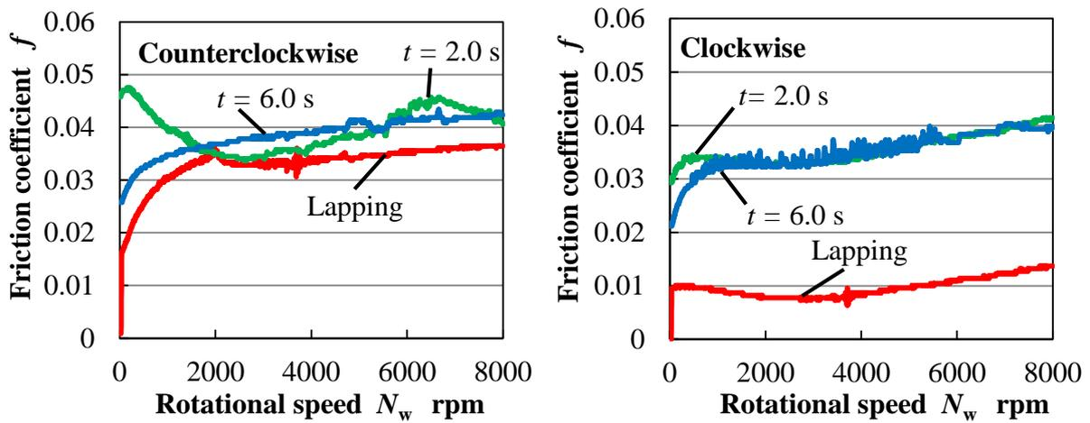
Fig.8 Relationship between rotational speed and friction coefficient
