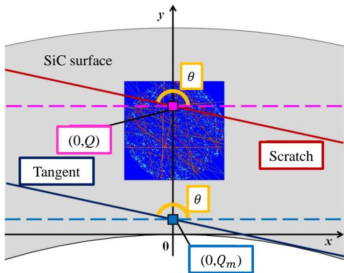
Fig.2 The analytical model of the scratches
