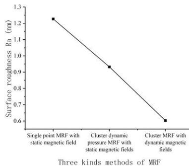
Fig 3 Effect of three MRF methods on the surface roughness of the workpiece
