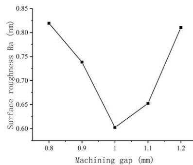
Fig 6 the effect of machining gap on the surface roughness of the workpiece
