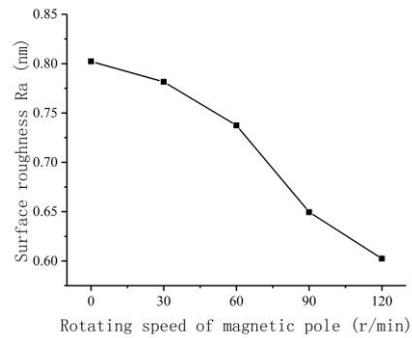
Fig 7 the influence of rotating speed of magnetic pole on the surface roughness of the workpiece
