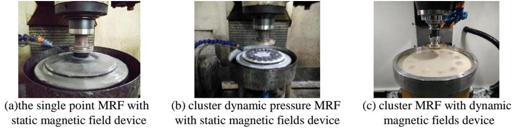
Fig 2 three kinds of MRF methods for polishing device.
