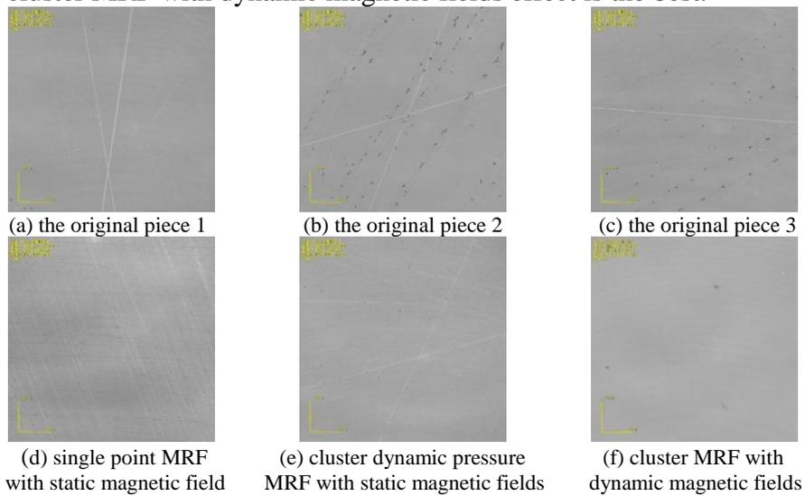
Fig 4 Surface morphology of workpiece with the same position before and after polishing by three MRF methods.
