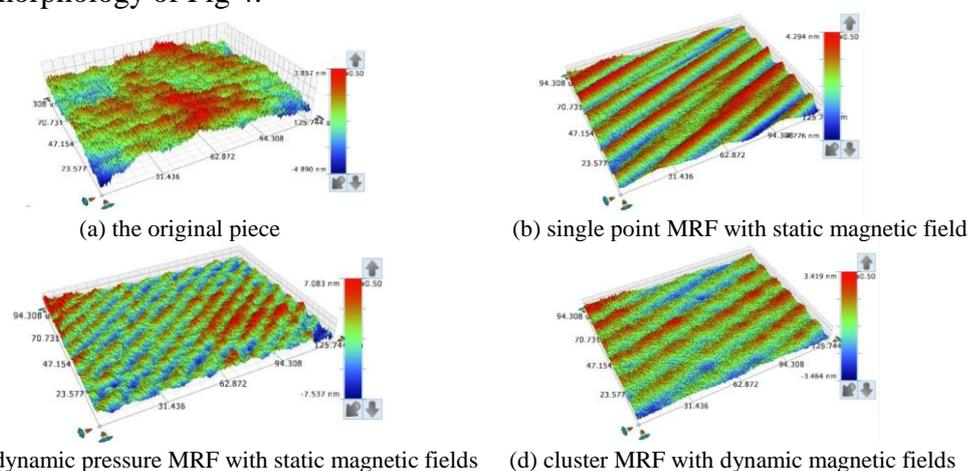
Fig 5 Surface morphology of workpiece before and after polishing by three MRF methods.
