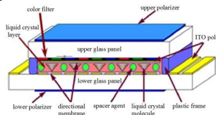
Fig. 1 Cross section chart of the inner screen of mobile phone
