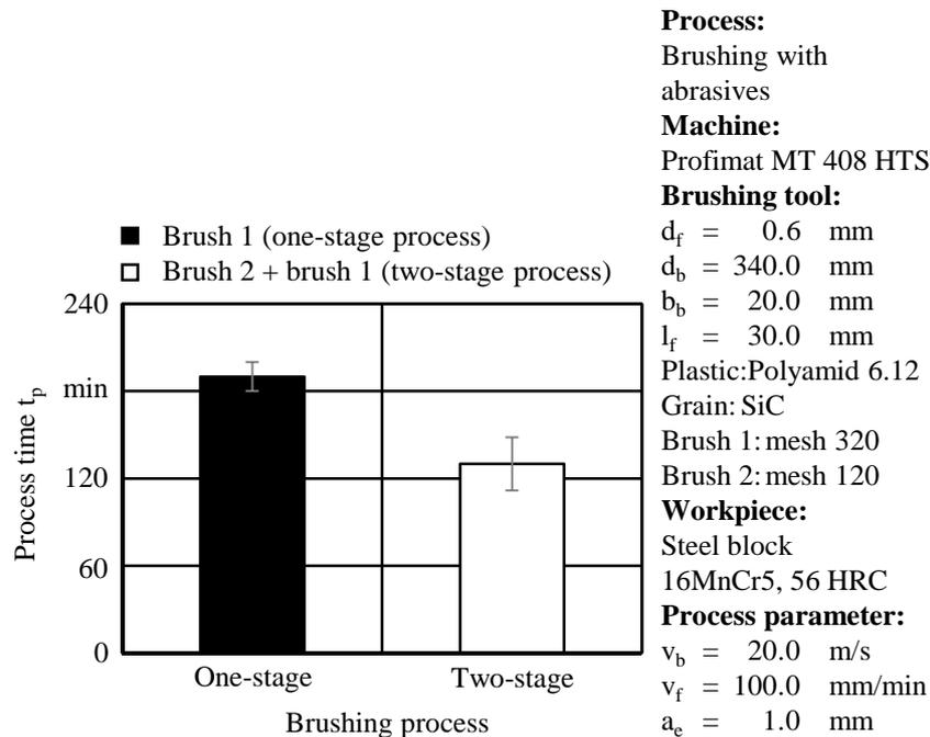
**Figure 6:** Process time  $t_p$  to manufacture a surface roughness of  $R_a < 0.1 \mu\text{m}$  for different brushing processes
