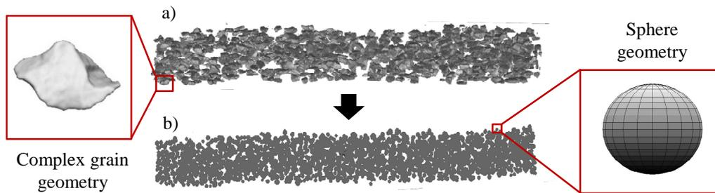
**Figure 2:** Filament structure analysis: a) voxel-graphic of the abrasive grains and b) approximation of the abrasive grains by spheres
