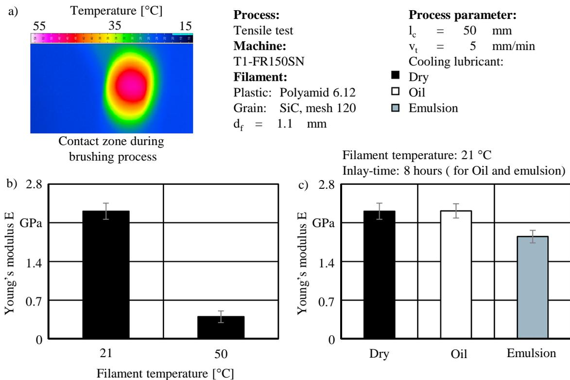
**Figure 4:** Influence of the contact zone temperature and the cooling lubricant on the Young's modulus
