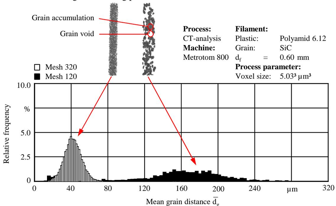
**Figure 3:** Mean grain distance  $\bar{d}_g$  in abrasive filaments
