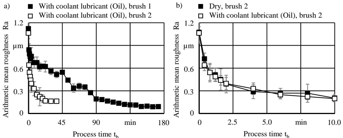
**Figure 5:** Brushing investigations: a) limiting roughness for the chosen brushes and b) roughness reduction for a dry and an cooled brushing process
