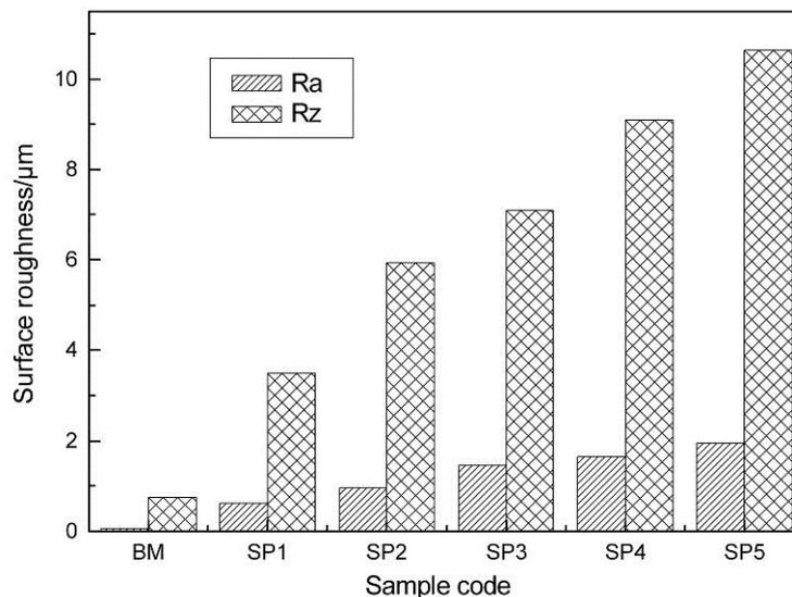
Fig. 1 Surface roughness of samples with untreated and SP treatments
