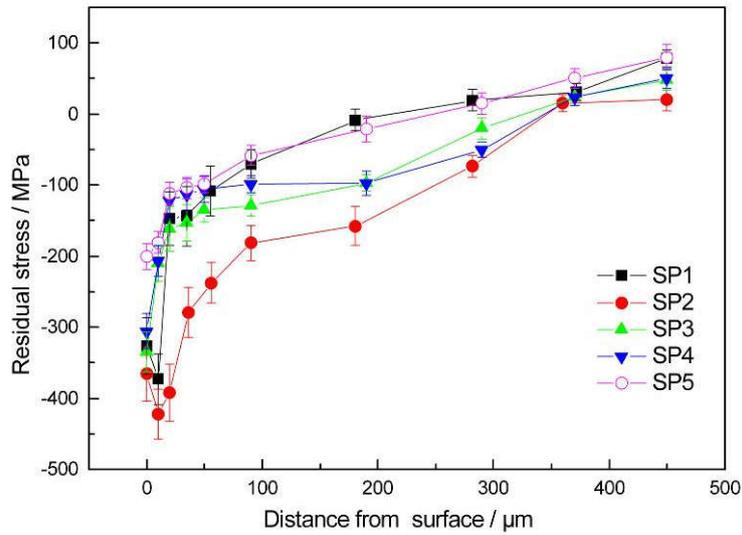
Fig. 3 Effect of SP treatments on surface residual stress of samples
