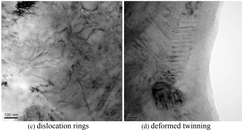
Fig. 4 TEM topography of high strength alloy with SP2 treatment at 10  $\mu\text{m}$  depth from surface
