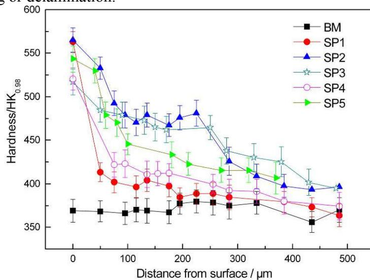
Fig. 2 Cross-hardness distribution of samples with untreated and SP treatments
