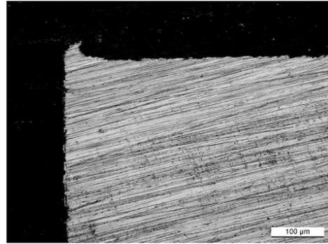
Fig. 4 Cross-sectional topography of burr
