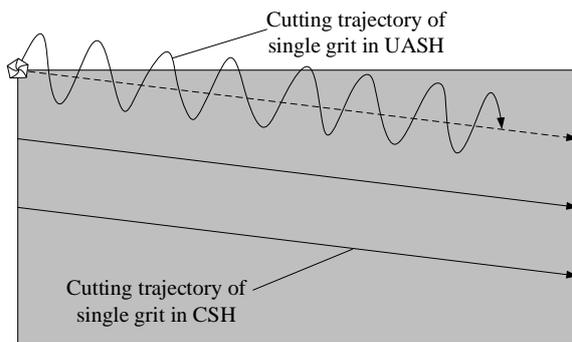
Fig. 6 Diagram of cutting trajectory of single grit
