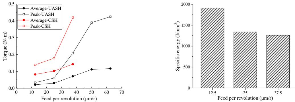
Fig. 7 Honing torque vs. feeding speed ( $n=2000\text{r/min}$ ,  $L=4\text{mm}$ )      Fig. 8 Specific energy vs. feeding speed ( $n=2000\text{r/min}$ ,  $L=4\text{mm}$ )
