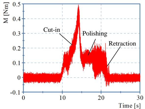
Fig. 2 Typical signal of honing torque ( $n=2000$ r/min,  $v_a=75$ mm/min, CSH)
