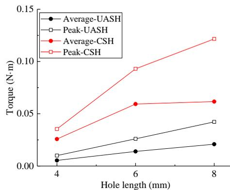
Fig. 9 Honing torque vs hole length ( $n=2000\text{r/min}$ ,  $f=17.5\mu\text{m/r}$ )
