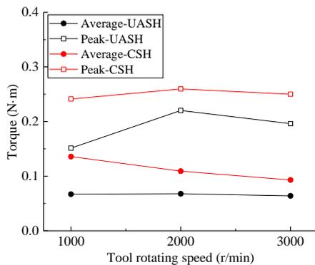
Fig. 5 Honing torque vs tool rotating speed ( $f=40\mu\text{m}/\text{r}$ ,  $L=4\text{mm}$ )
