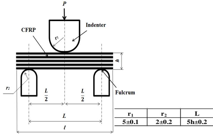
Fig. 4 Three-point bending test
