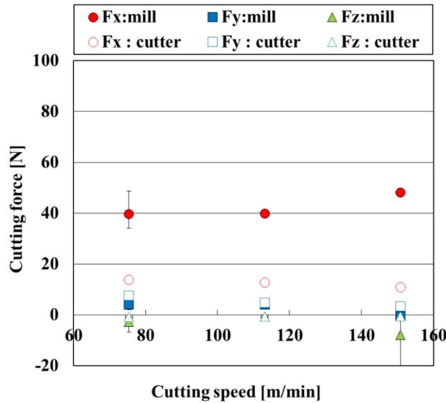
Fig. 8 Cutting forces  $F_x$ ,  $F_y$ ,  $F_z$  ( $f=0.065\text{mm/rev}$ ,  $b=0.6\text{mm}$ )
