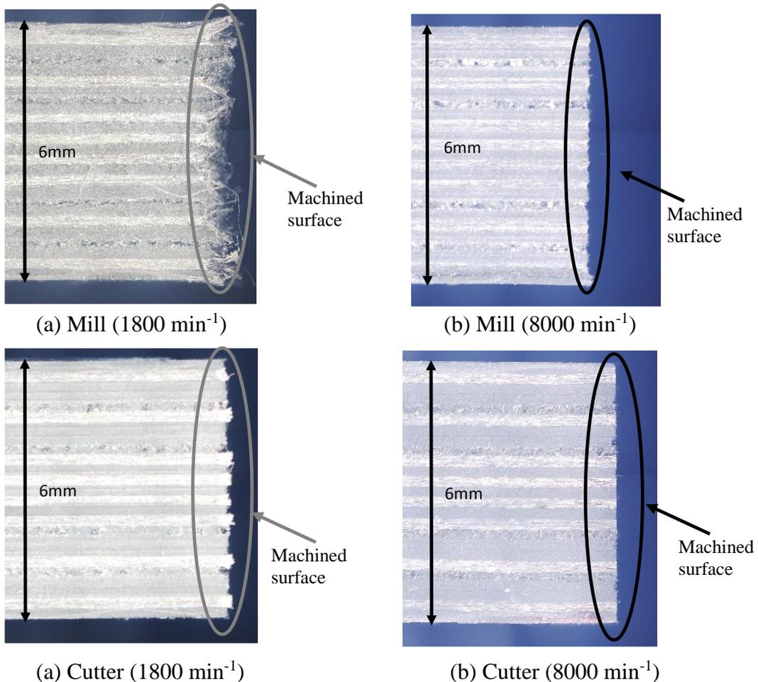
Fig. 7 Photograph of machined surface ( $f=0.065\text{mm/rev}$ ,  $b=0.6\text{mm}$ )
