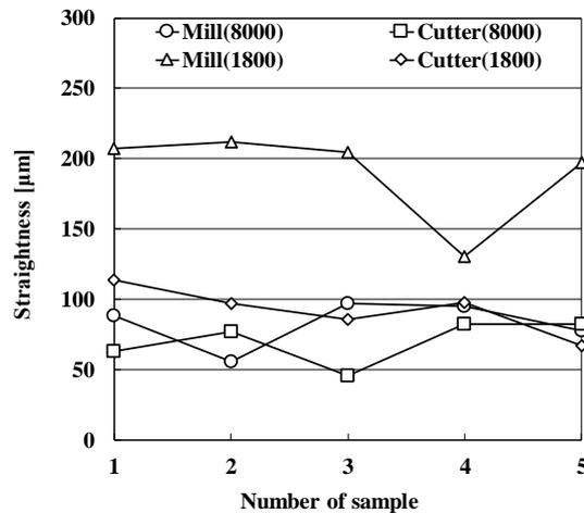
Fig. 5 Straightness of machined surface ( $f=0.065 \text{ mm/rev}$ ,  $b=0.6 \text{ mm}$ )
