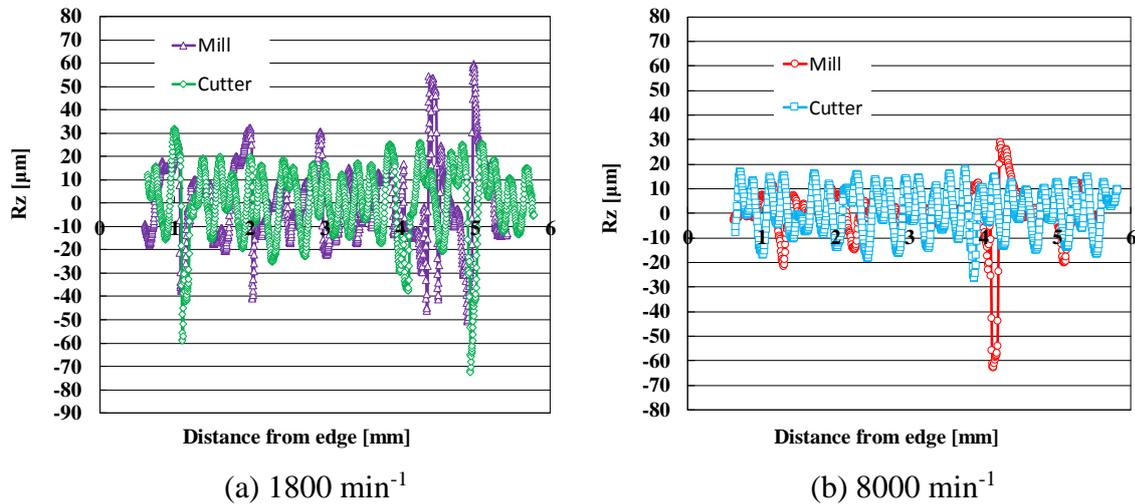
Fig. 6 Maximum height roughness of machined surface  $R_z$  ( $f=0.065\text{mm/rev}$ ,  $b=0.6\text{mm}$ )
