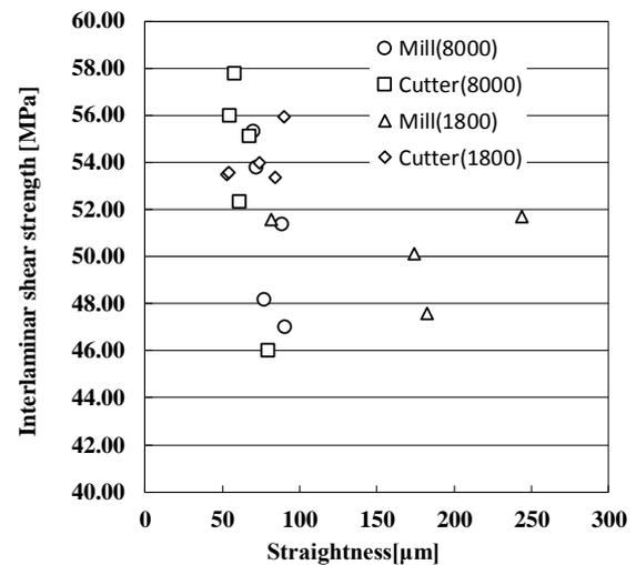
Fig. 9 Interlaminar shear strength ( $f=0.065\text{mm/rev}$ ,  $b=0.6\text{mm}$ )
