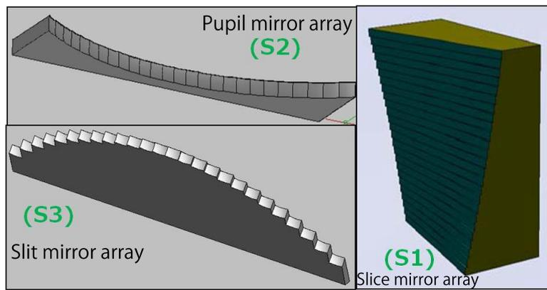
Figure 2. Three types of mirror arrays for SWIMS-IFU, Slice mirror array (S1), Pupil mirror array (S2) and Slit mirror array (S3) [1].
