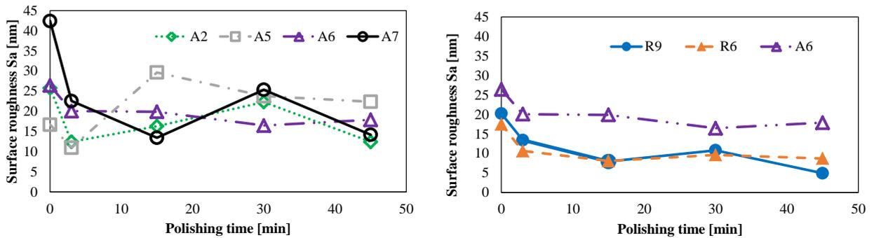
(a) Conventional aluminum (A2, A5, A6, A7) (b) Melt span aluminum alloy (R9, R6).
