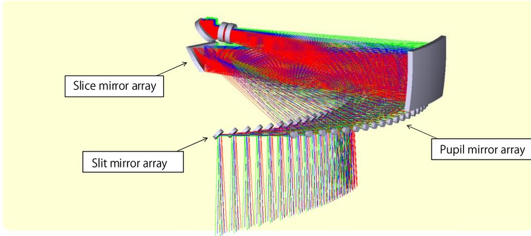
Figure 1. Optical design of Integral Field Unit (IFU) for Simultaneous-color Wide-field Infrared Multi-object Spectrograph (SWIMS) [1].
