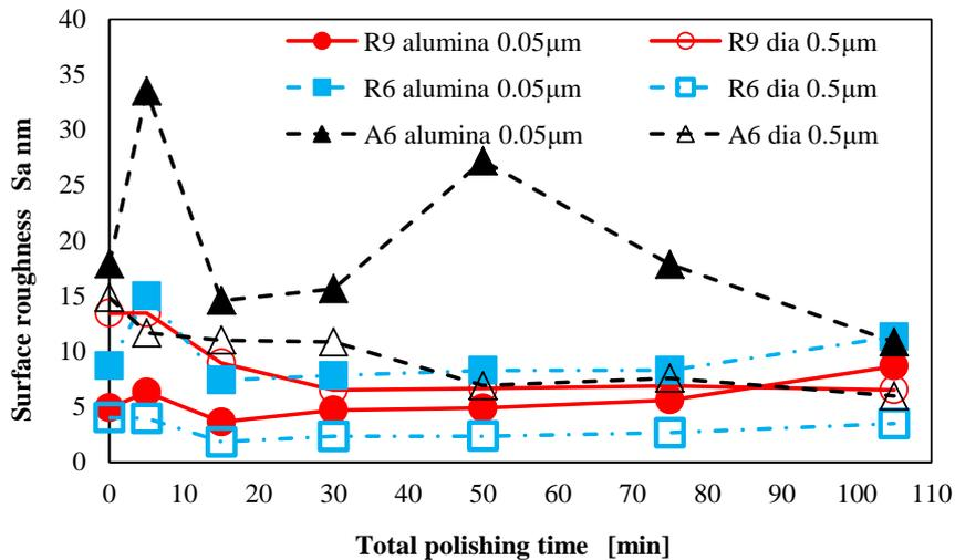
Figure 7. Surface roughness results according to the polishing time in polishing R9, R6 and A6.
