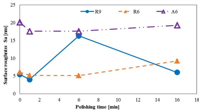
(a) Surface roughness results according to the polishing time
