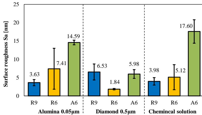
Figure 6. Comparison between 3 different polishing slurry in polishing R9, R6 and A6
