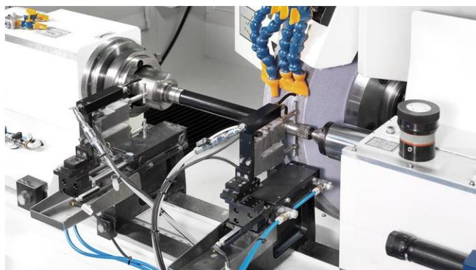
Fig. 1: Outer diameter (OD) cylindrical grinding process [[www.danobatgroup.com](http://www.danobatgroup.com)].
