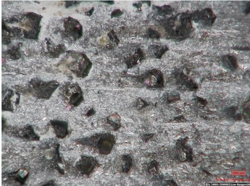
Fig.7 surface of the wheel before electrolysis
