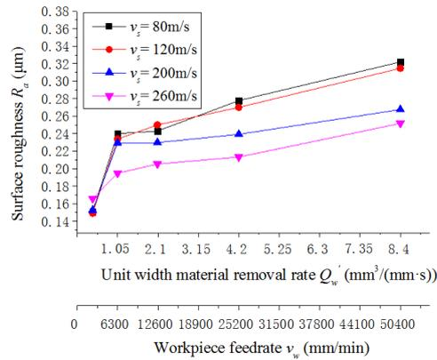
Fig.4 Effect of material removal rate per unit width on surface roughness of grinding workpiece
