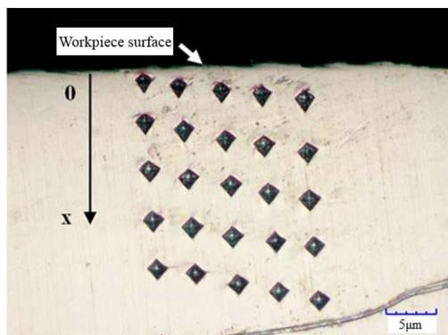
Fig.5 Microhardness measuring point
