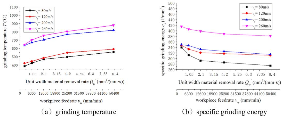
Fig.3 Effect of material removal rate per unit width on specific grinding energy
