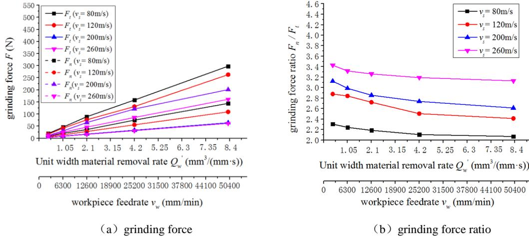
Fig.2 Effect of material removal rate per unit width on grinding force and grinding force ratio
