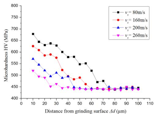
Fig.6 Microhardness distribution on the surface of grinding workpiece
