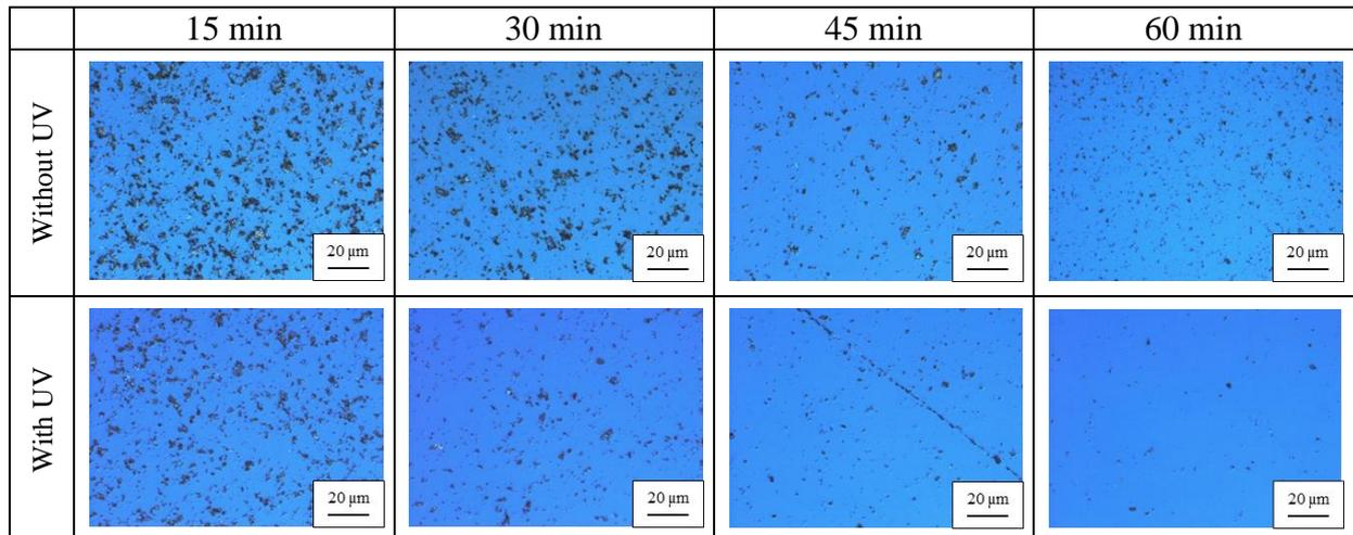
Fig. 4 Optical microscopic images of workpiece surface after grinding
