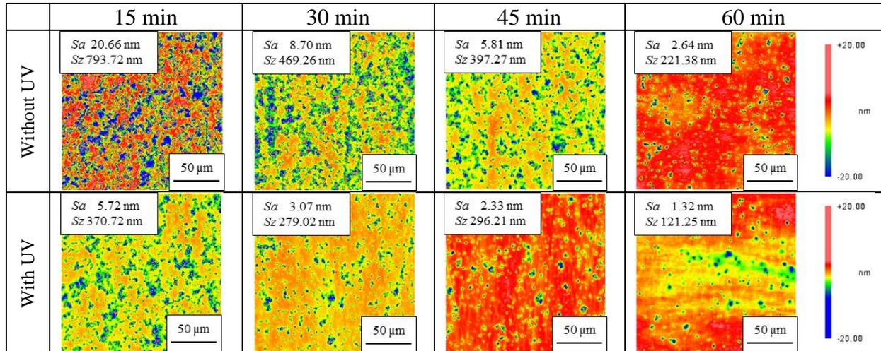
Fig. 5 Interferometric images of workpiece surface after grinding
