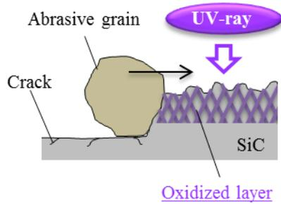
Fig. 1 Schematic diagram of UV-assisted grinding
