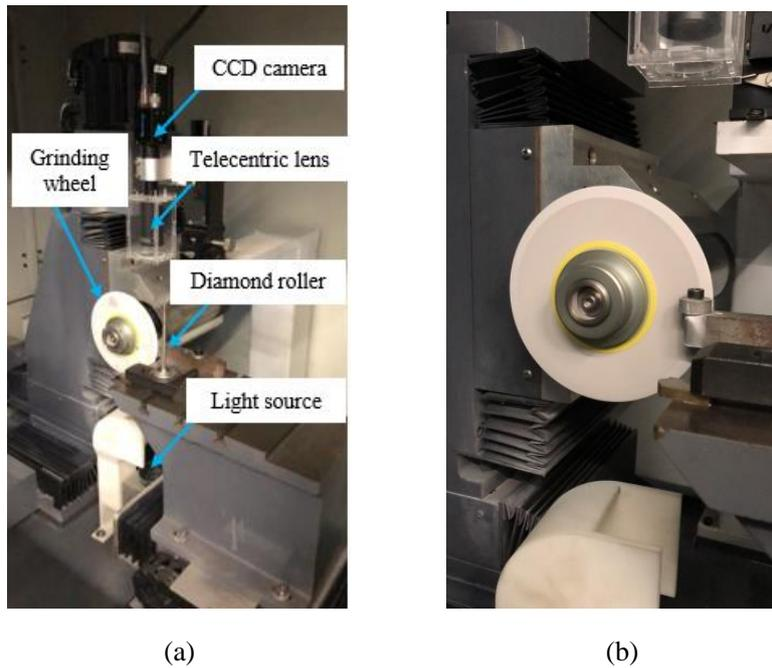
Fig. 7 Experiment platform: (a)Self-developed profile grinding testbed; (b) Wheel and dresser in ressing.
