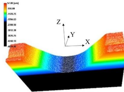
Fig.4 3D profiler measurement result of duplicated profile
