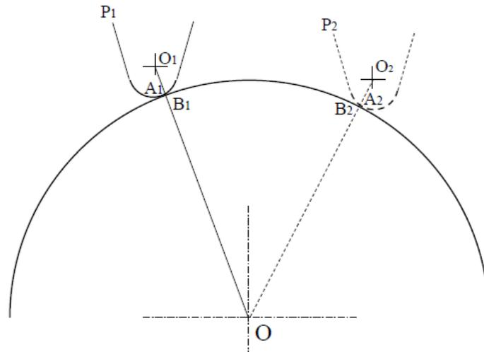
Fig. 6 Schematic diagram for diamond roller dressing of grinding wheel
