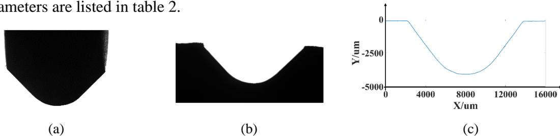
Fig. 5 The results of three measurement methods for measuring of wheel edge profile: (a)In-situ visual measurement of wheel profile;(b)In-situ visual measurement of duplicated wheel profile; (c) Profiler measurement of duplicated wheel profile.
