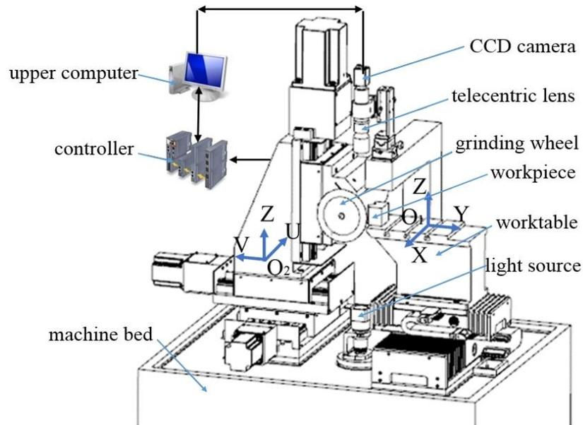
Fig. 1 Structure diagram for in-situ vision measurement of wheel profile in profile grinding
