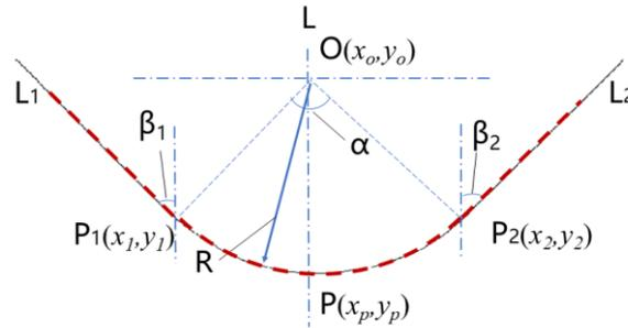
Fig. 2 Edge extraction and curve fitting for wheel profile
