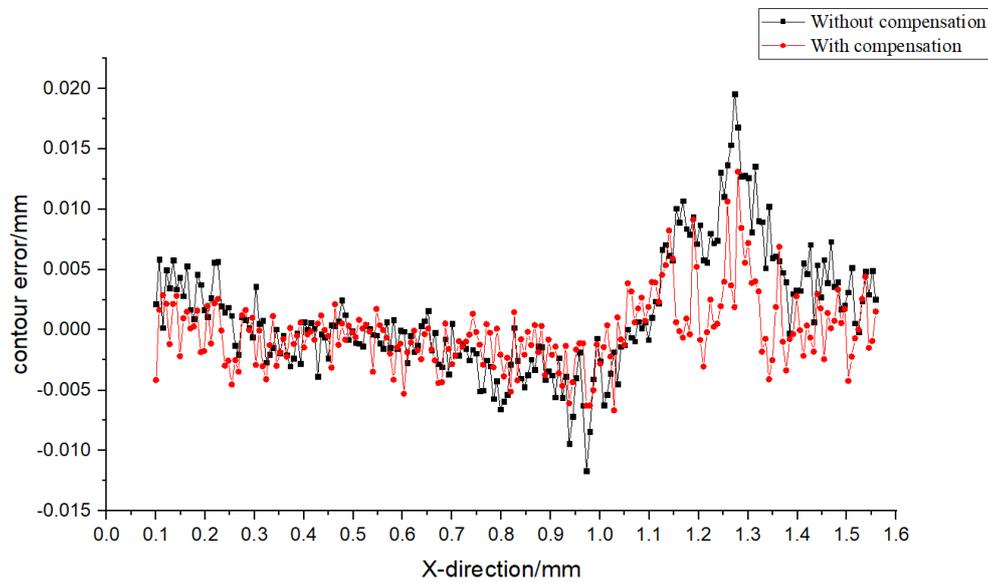
Fig. 8 Contour error distribution of grinding wheel before and after compensation
