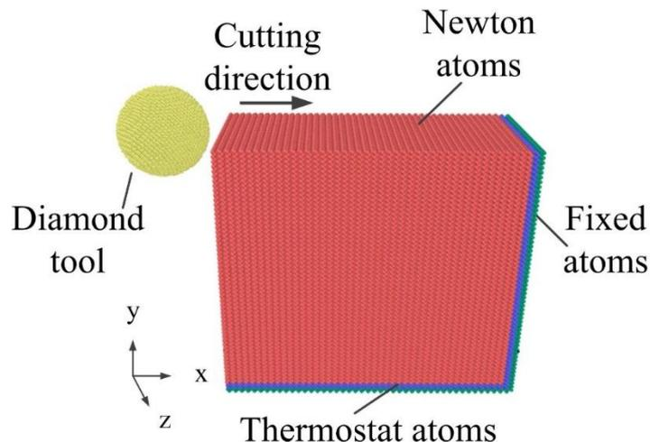
**Fig. 1.** Schematic model of the nanometric scratching simulation
