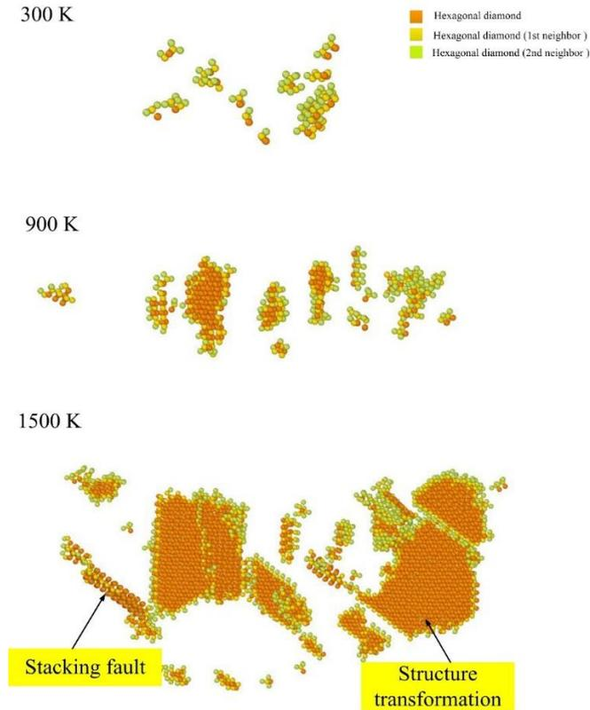
**Fig. 4** Subsurface defects of structure transformation distribution in substrate of SiC.
