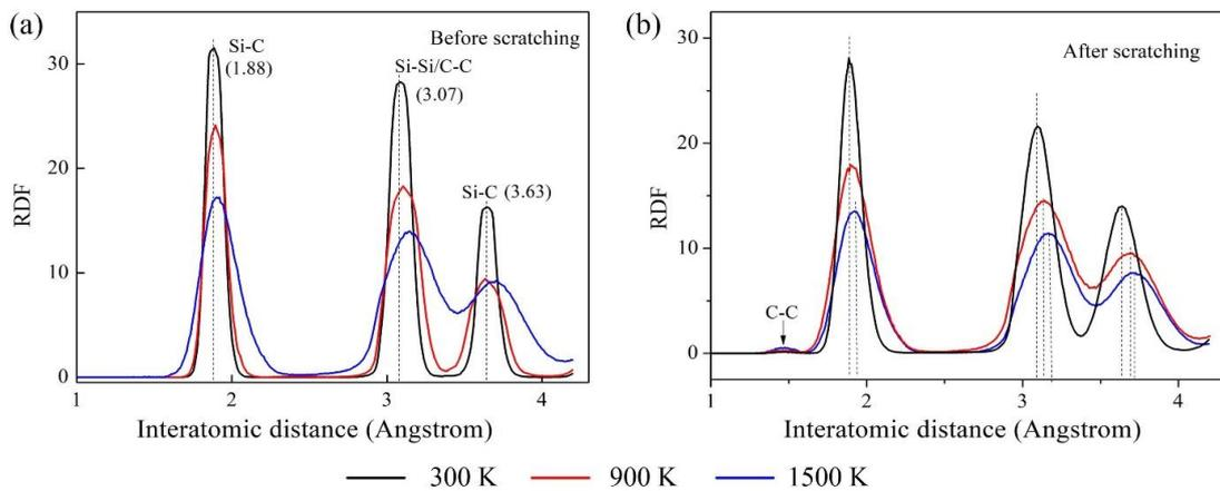
**Fig.3** Radial pair distribution function at different temperature for SiC.
