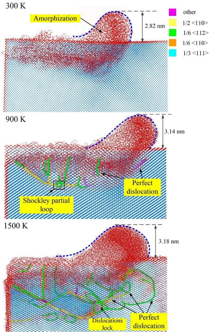
**Fig. 2** Snapshots of surface and subsurface defects during scratching process.
