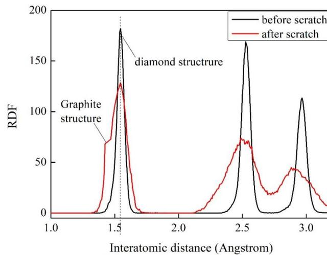
**Fig. 6.** The Radial pair distribution function at temperature of 1500 K for diamond.
