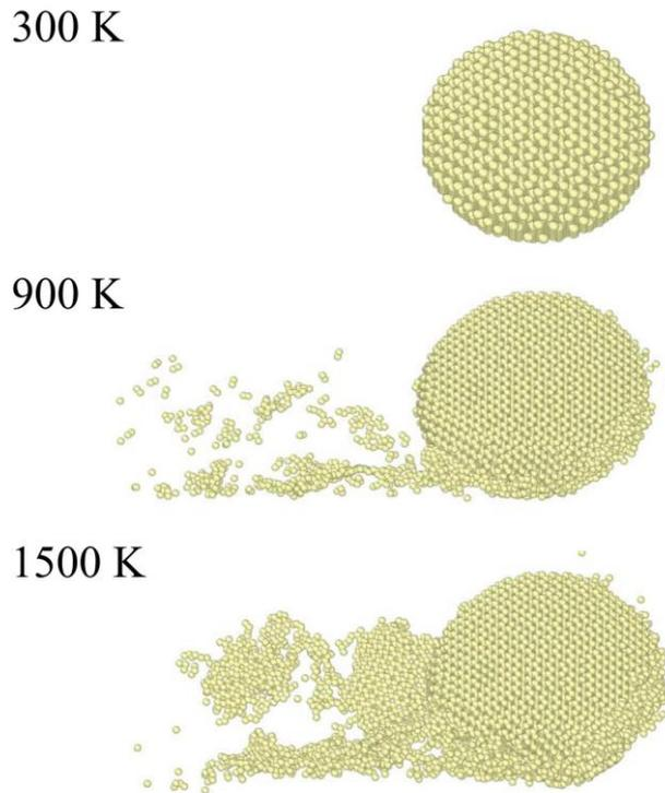
**Fig. 5.** The wear state of diamond tool after scratching at each temperature.
