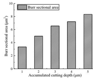
Fig. 13 Burr sectional areas vs. accumulated cutting depths ( $v_s=0.1\text{m/s}$ ,  $a_e=5\mu\text{m}$ ,  $a_p=1\mu\text{m}$ ,  $\theta=0$ )
