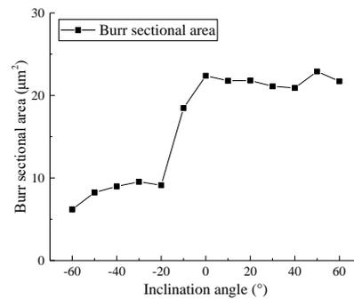
Fig. 16 Burr sectional areas under different inclination angles ( $v_s=0.1\text{m/s}$ ,  $a_e=5\mu\text{m}$ ,  $a_p=5\mu\text{m}$ )
