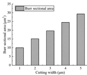
Fig. 9 Burr sectional areas under different cutting widths ( $v_s=0.1\text{m/s}$ ,  $a_p=5\mu\text{m}$ ,  $\theta=0$ )
