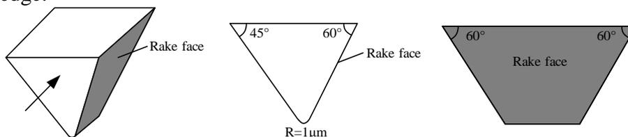
Fig. 4 Diagram of grit shape
