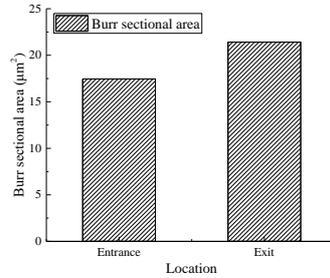
Fig. 8 Burr sectional areas at entrance and exit ( $v_s=0.1\text{m/s}$ ,  $a_p=5\mu\text{m}$ ,  $a_e=5\mu\text{m}$ ,  $\theta=0$ )
