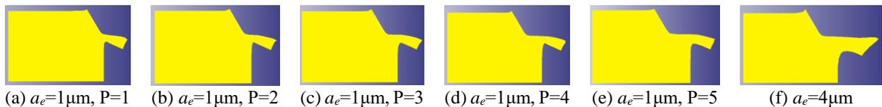
Fig. 11 Burr sectional topography under different cutting parameters ( $v_s=0.1\text{m/s}$ ,  $a_p=5\mu\text{m}$ ,  $\theta=0$ )
