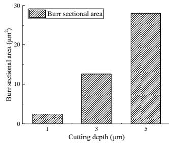
Fig. 12 Burr sectional areas under different cutting depths ( $v_s=0.1\text{m/s}$ ,  $a_e=5\mu\text{m}$ ,  $\theta=0$ )
