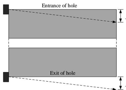
Fig. 3 Cutting states at the entrance and exit of holes
