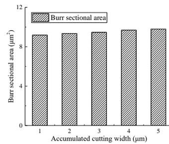
Fig. 10 Burr sectional areas vs. accumulated cutting widths ( $v_s=0.1\text{m/s}$ ,  $a_p=5\mu\text{m}$ ,  $a_e=1\mu\text{m}$ ,  $\theta=0$ )
