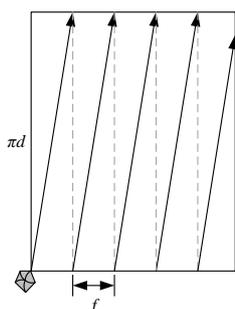
Fig. 2 Diagram of unfolded workpiece surface
