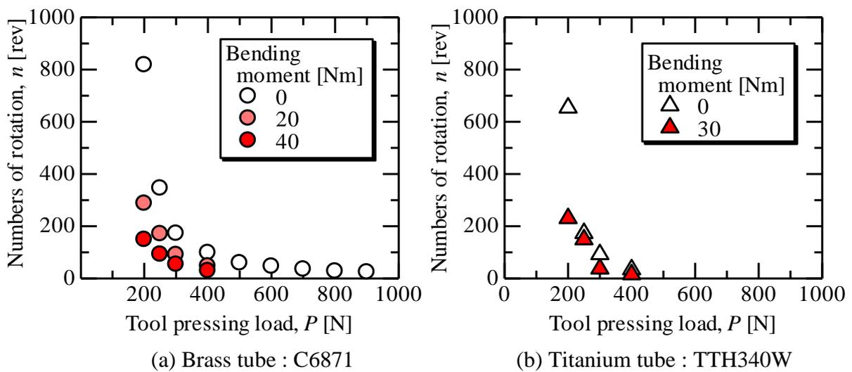
Fig. 10 Relationship between bending moment and numbers of rotation
