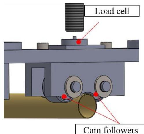
Fig. 4 Tube bending unit
