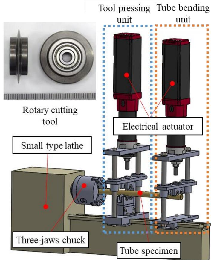
Fig. 2 Experimentl setup for cut-off tube
