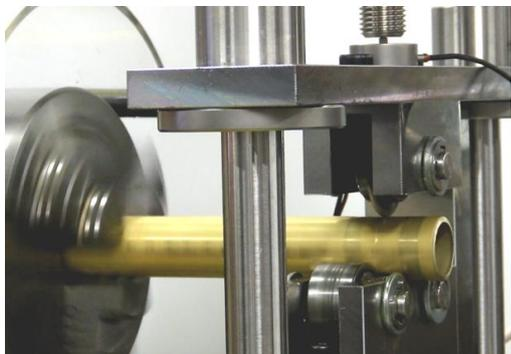
Fig. 6 Cut-off the tube specimen
