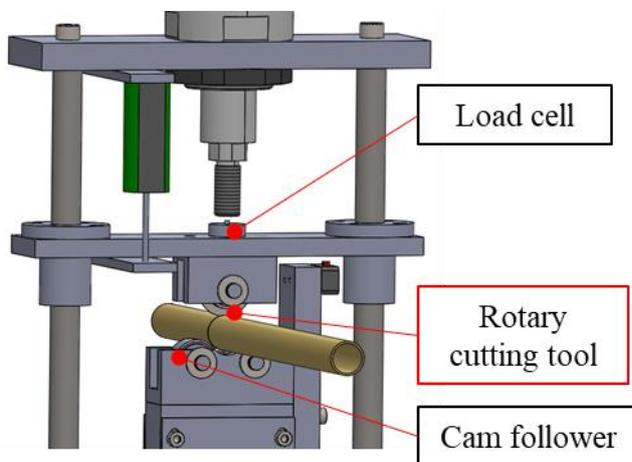
Fig. 3 Tool pressing unit
