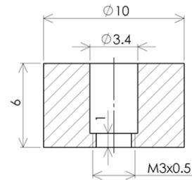
Fig. 2 Shape of the test piece prepared for evaluating the strength of internal threads
