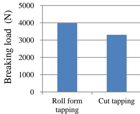
Fig. 10 Comparison in strength of the internal threads machined with a rolled tap and a cutting tap.
