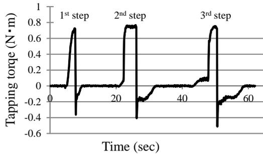
Fig. 7 An example of the change in tapping torque in three-step feed
