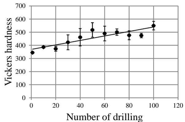
Fig. 4 Relationship between the number of drilling and the Vickers hardness of pilot hole surface.
