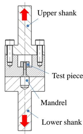
Fig. 3 Method for evaluating the strength of internal threads
