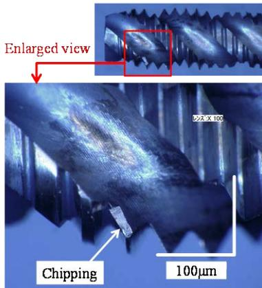
Fig. 9 The microscope image of the cutting edge of cutting tap after the first tapping process.
