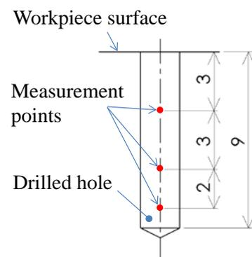
Fig. 1 Measurement points of Vickers hardness
