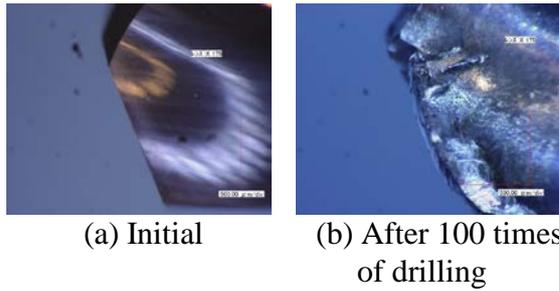
Fig. 5 Microscope images of the cutting edge of drill before and after 100 times of drilling
