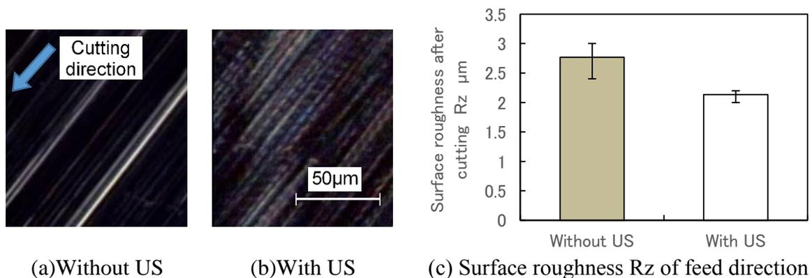
Fig.6 Surface conditions and surface roughness of hardened steel after rotary cutting
