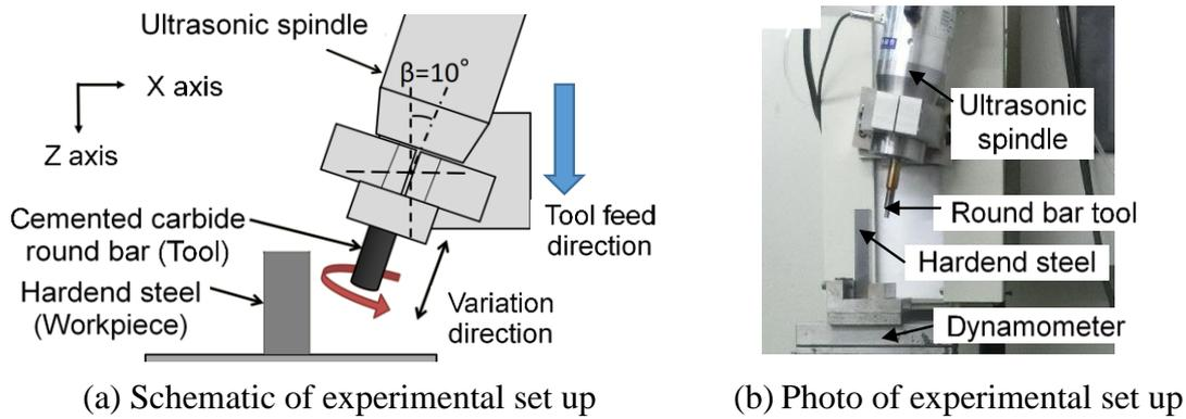
Fig.7 Outline of linear R groove machining experiment by ultrasonic rotary cutting
