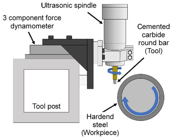
(a) Schematic of experimental set up
