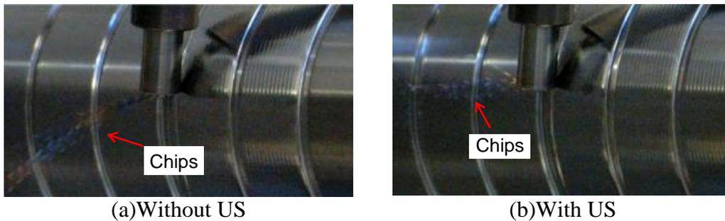
Fig.4 Difference of chip discharge direction during rotary cutting
