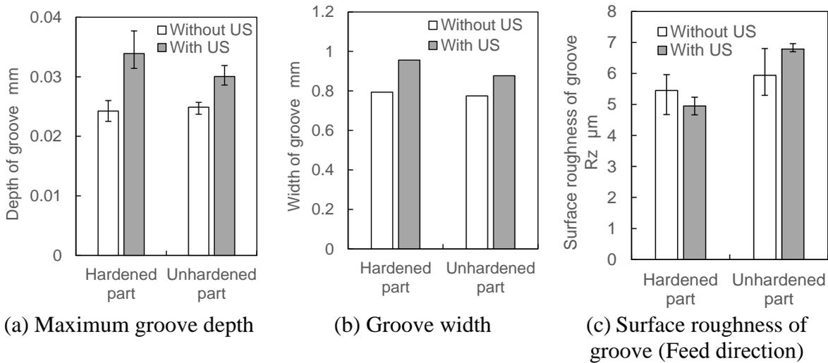
(a) Maximum groove depth (b) Groove width (c) Surface roughness of groove (Feed direction)
