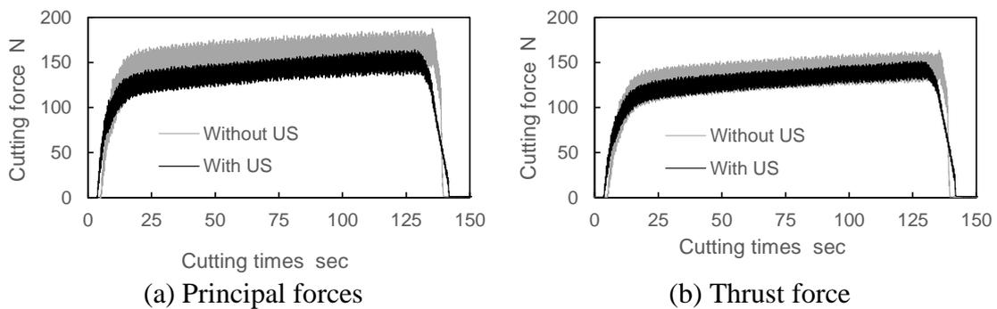
Fig.5 Cutting force during rotary cutting (2nd pass)
