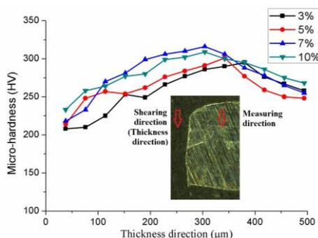
Fig.7 Micro-hardness of shear direction
