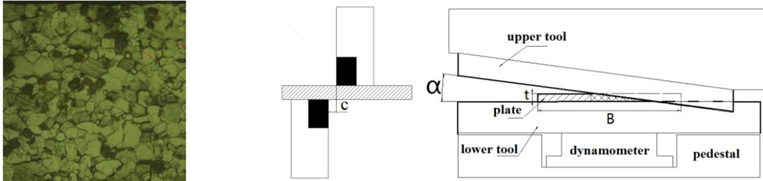
Fig.1 Microstructure of electrical steel Fig.2 Oblique shear principle:(A) Sectional view ;(b) Front view
