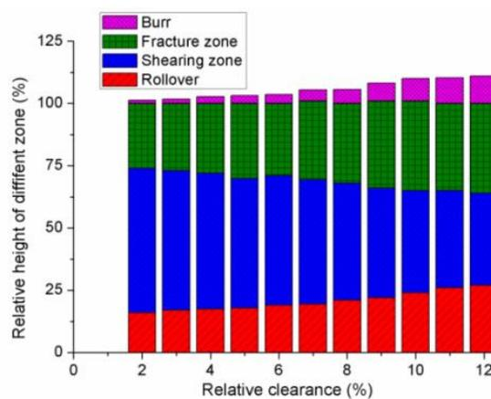
Fig 5. The height of each morphology characteristic under different shear clearances
