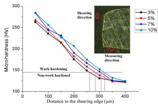
Fig.8 Micro-hardness curve Distance shear edge
