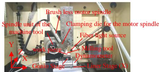
Fig. 3 Machine tool in the milling test
