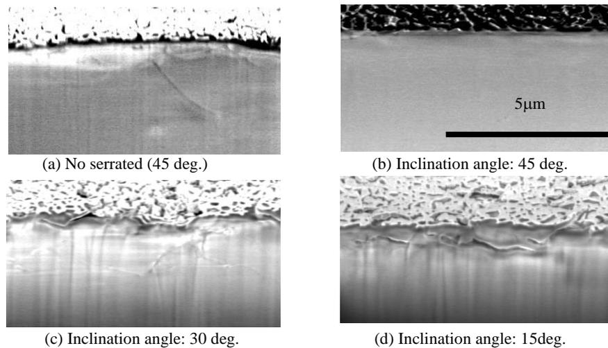
Fig.7 Cross section under the machined surface
