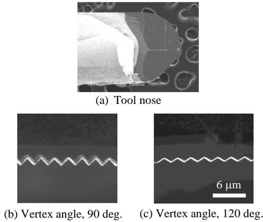
Fig. 1 Serrated SCD ball endmill [3]
