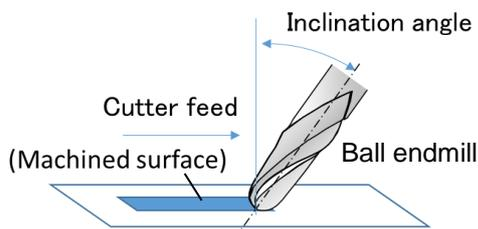
Fig. 4 R0.5 SCD ball endmill in the milling test
