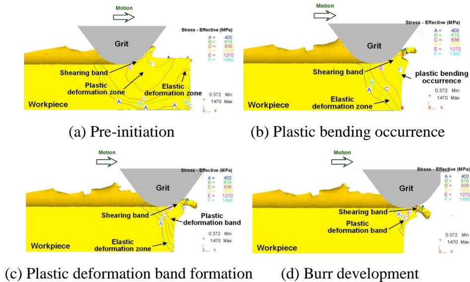
Fig. 2. The procedures of the exit burr formation
