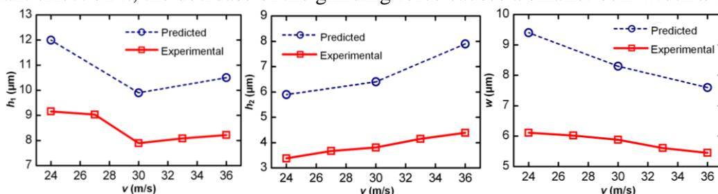
Fig. 4. Effects of the grinding speed on exit burr sizes
