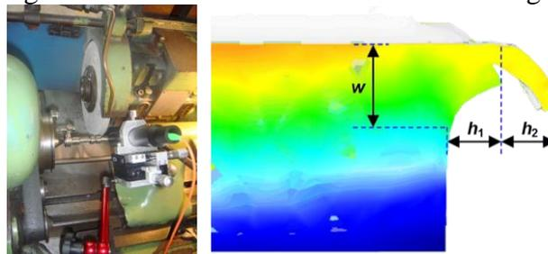
Fig. 3. (a) Experimental setup, (b) Measurement of burr sizes.
