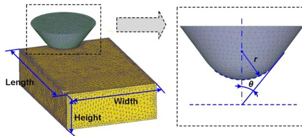
Fig. 1. The grit and workpiece for the single grit grinding simulation
