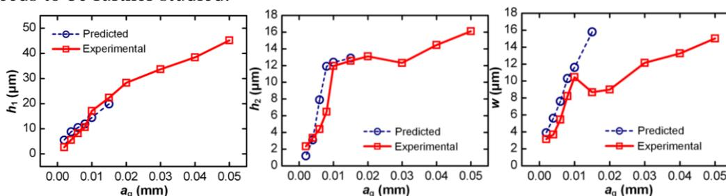
Fig. 5. Effects of the grinding depth on exit burr sizes
