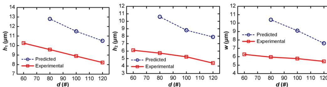
Fig. 6. Effects of the wheel granularity (grit size) on exit burr sizes
