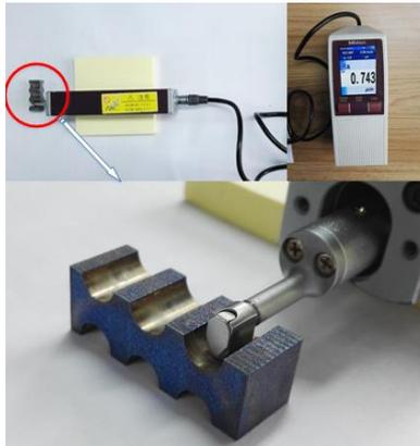
Fig. 7 Measurement of surface roughness of the drilled holes
