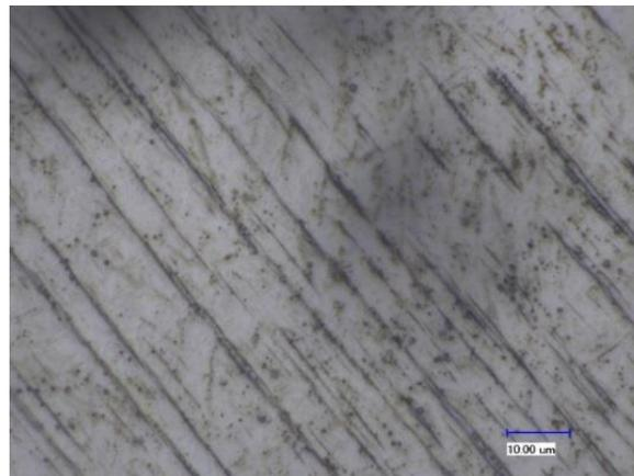
Fig. 1 Microstructure of 3D-printed Ti6Al4V (3000X)
