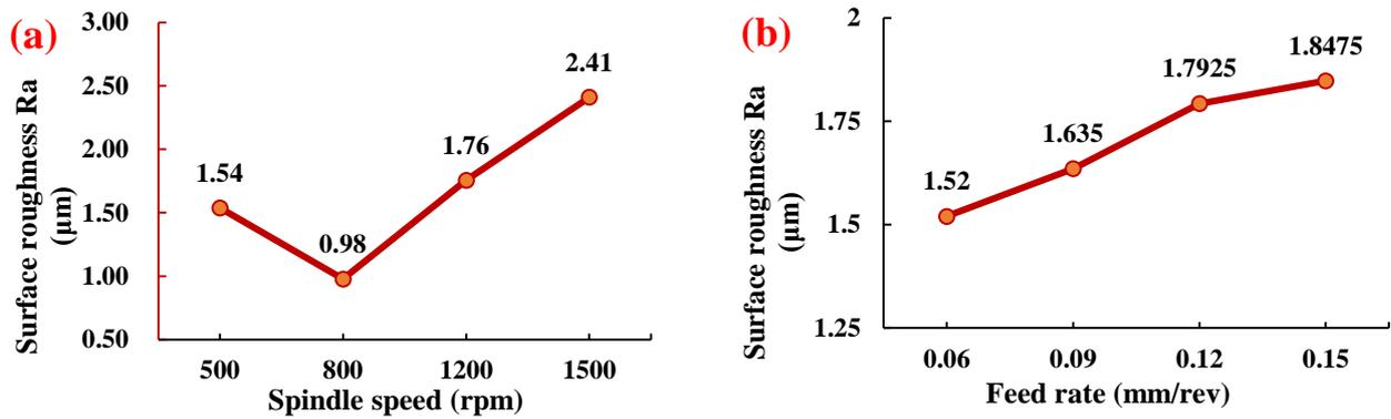
Fig. 8 Surface roughness results of drilling tests: (a) Ra at various cutting speed; (b) Ra at various feed rate
