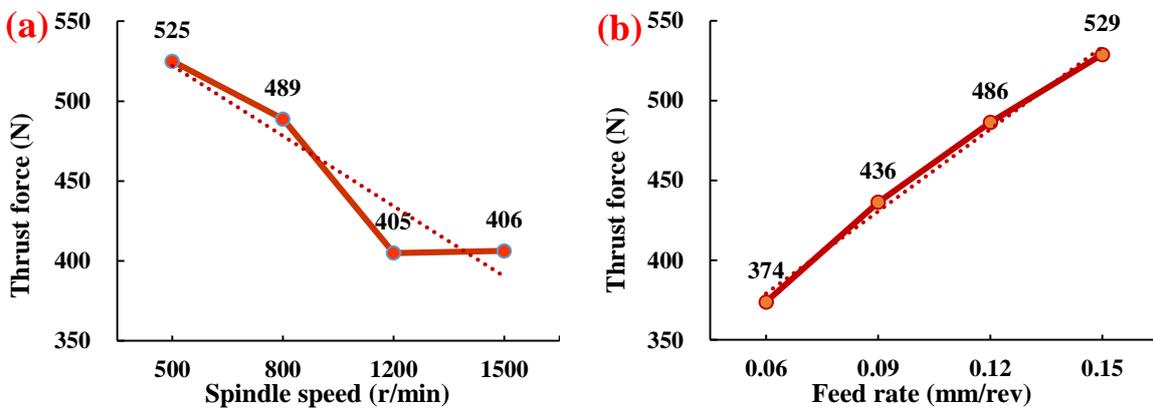
Fig. 5 Thrust forces results of drilling tests: (a) Thrust forces at various cutting speed; (b) Thrust forces at various feed rate
