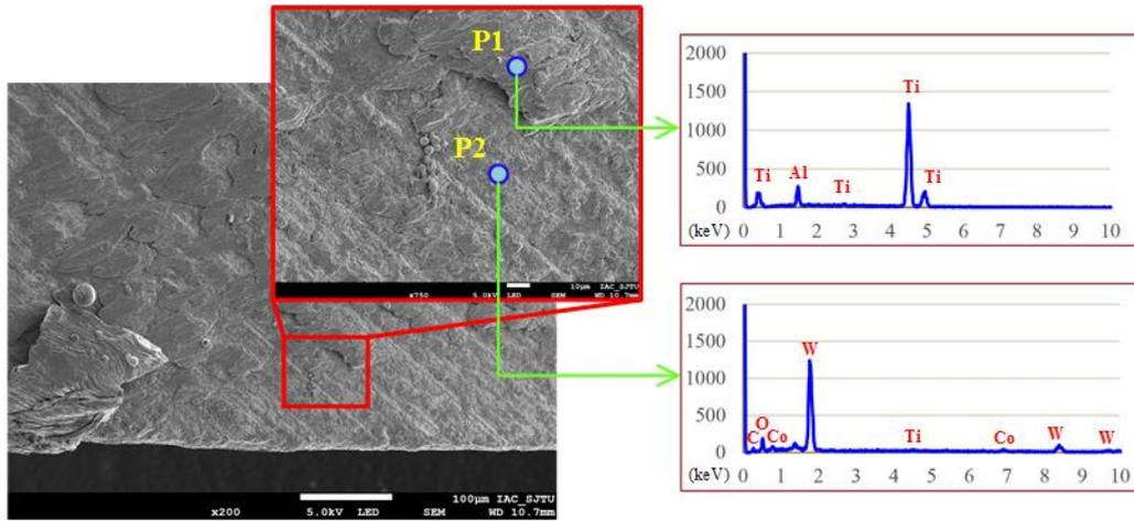
Fig. 4 EDS analysis on tool's rake face
