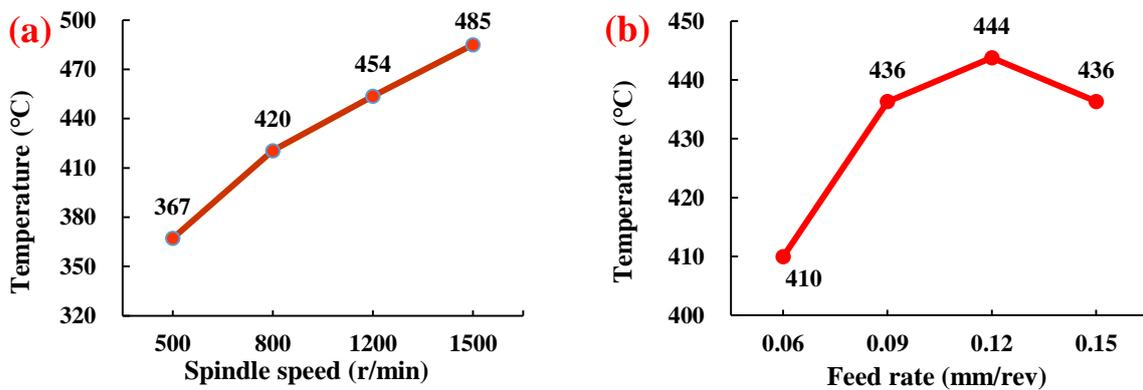
Fig. 6 Drilling temperature results of drilling tests: (a) Drilling temperature at various cutting speed; (b) Drilling temperature at various feed rate
