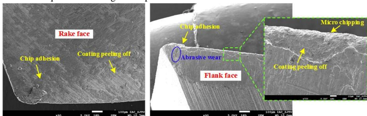
Fig. 3 SEM of the rake face and flank face of the worn tool
