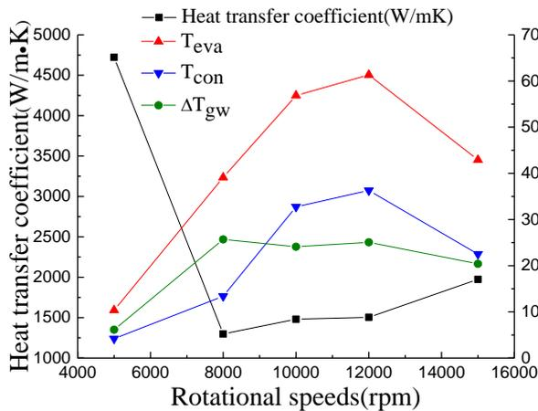
Fig. 6 Temperature and heat transfer coefficient vs. different rotational speeds
