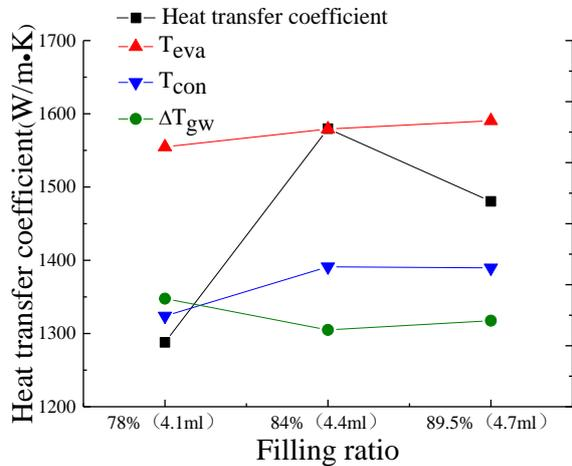
Fig. 4 Temperature and heat transfer coefficient vs. different filling ratios
