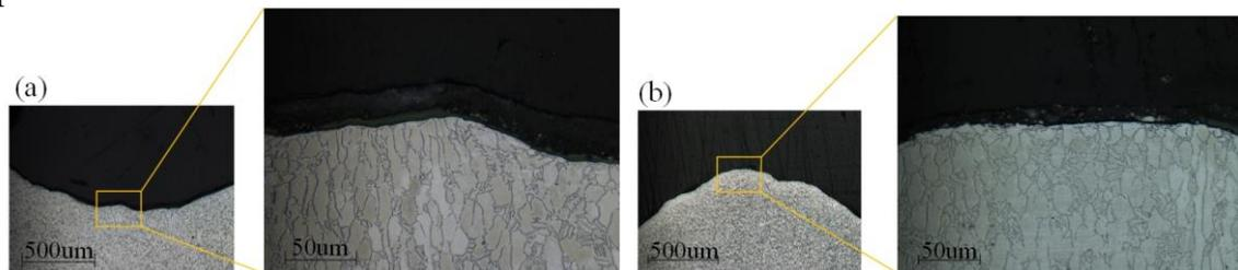
Fig. 9 The metallographic structure of the workpiece after grinding:
