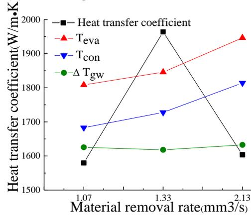
Fig. 2 Temperature and heat transfer coefficient vs. different material removal rates
