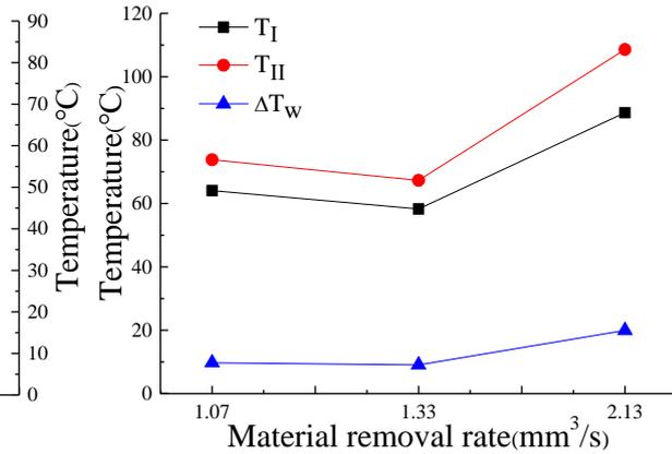
Fig. 3 Temperature of ground surface vs. different material removal rates
