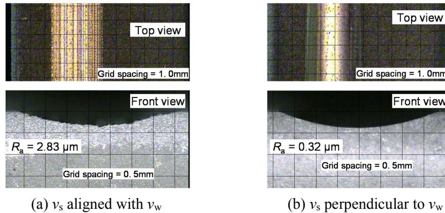
Fig. 5 Microscopic pictures of ground grooves
