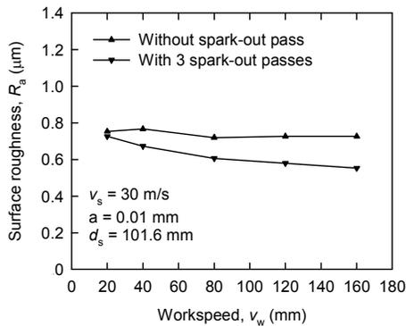
Fig. 3 Effects of workspeed on  $R_a$
