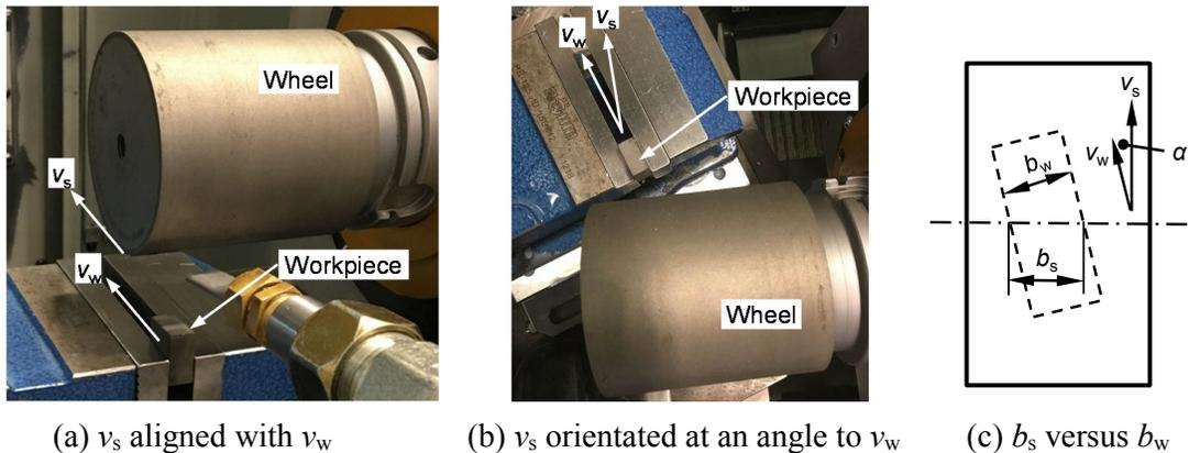
Fig. 1 Relationship between the directions of wheel speed and workspeed
