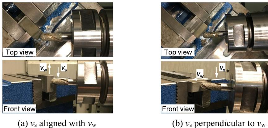
Fig. 2 Setup pictures of the small wheel
