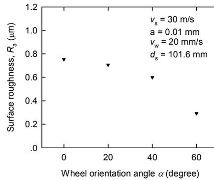
Fig. 4 Effects of orientation angle on  $R_a$
