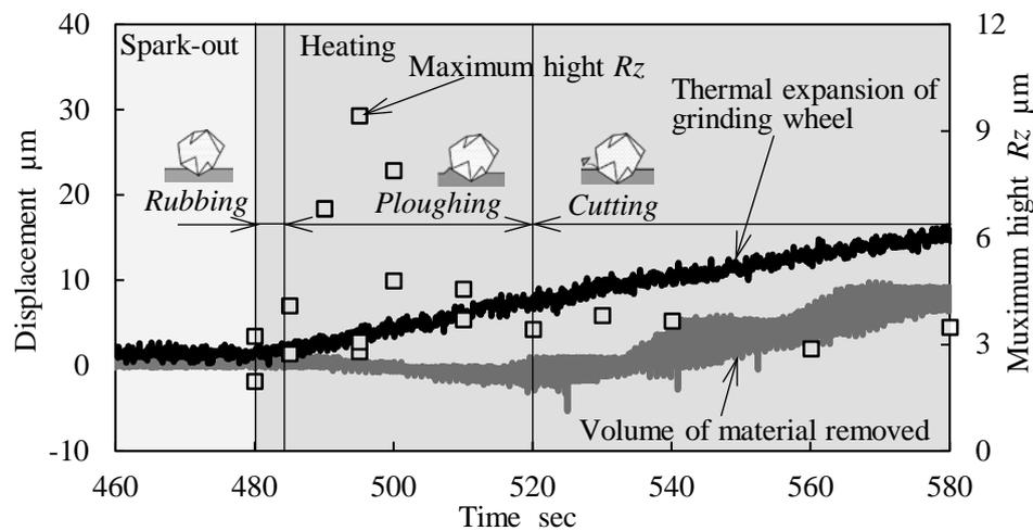
Fig. 5 Measured results of surface roughness
