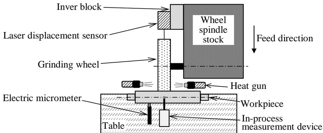
Fig.1 Schematic diagram of cylindrical grinding machine equipped with measuring devices
