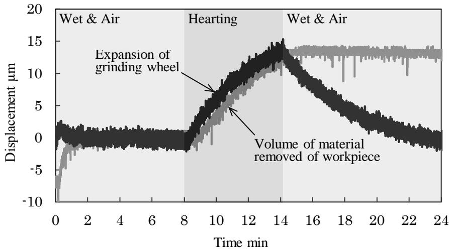
Fig.3 Thermal expansion of grinding wheel in wet grinding
