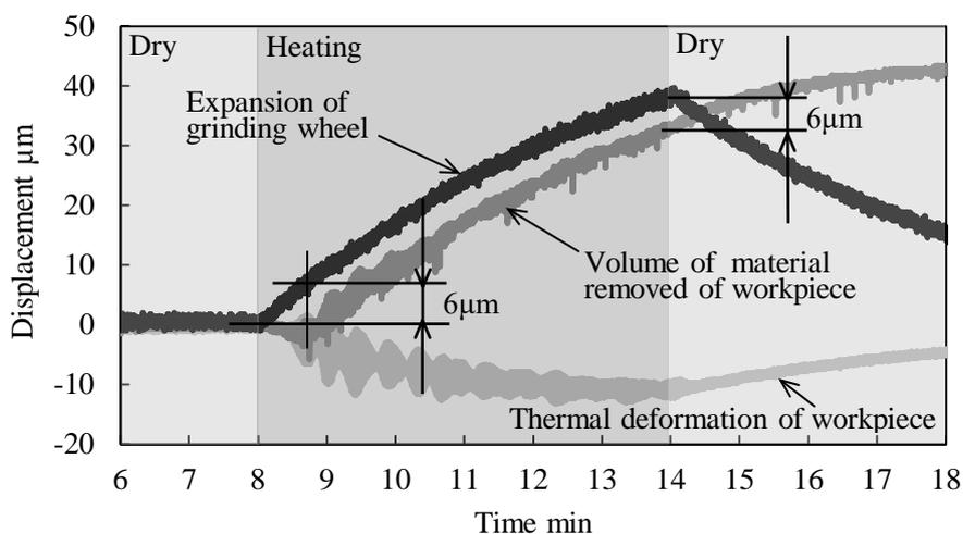
Fig.2 Thermal expansion of grinding wheel in dry grinding
