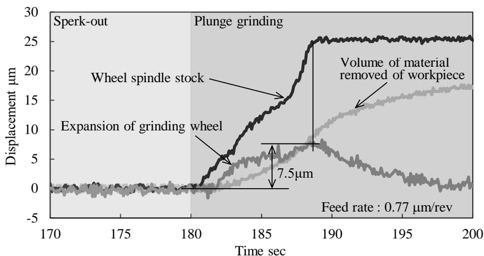
Fig.6 Relation between feed rate and volume of material removed of workpiece
