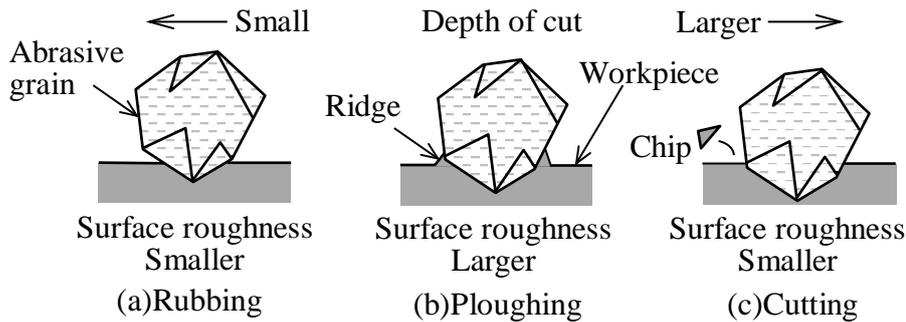
Fig.4 Schematic diagram of rubbing, ploughing and cutting
