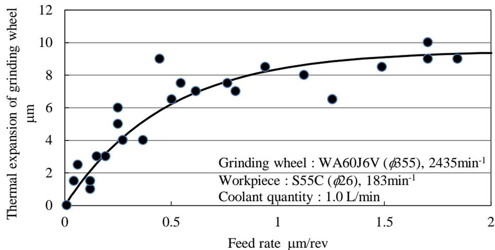
Fig. 7 Relation between feed rate and thermal expansion of grinding wheel
