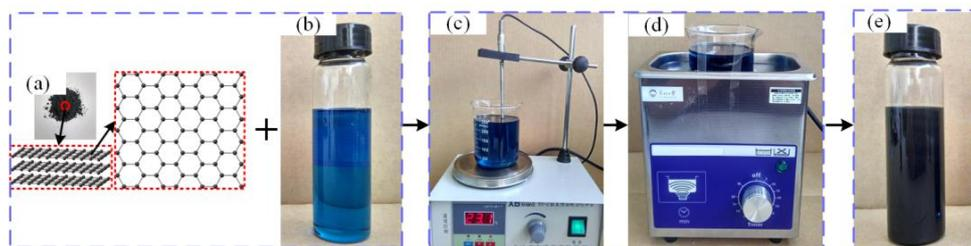
**Fig. 1.** This preparation process of graphene nanofluid ((a) the few-layer graphene, (b) pure LB200, (c) magnetic stirrer, (d) ultrasonic dispersion instrument and (e) graphene nanofluid)
