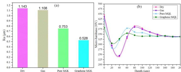
**Fig. 5.** (a) The surface roughness and (b) the tendency of micro-hardness
