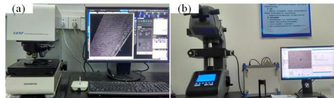
**Fig. 3.** (a) Laser confocal microscope and (b) micro-hardness tester
