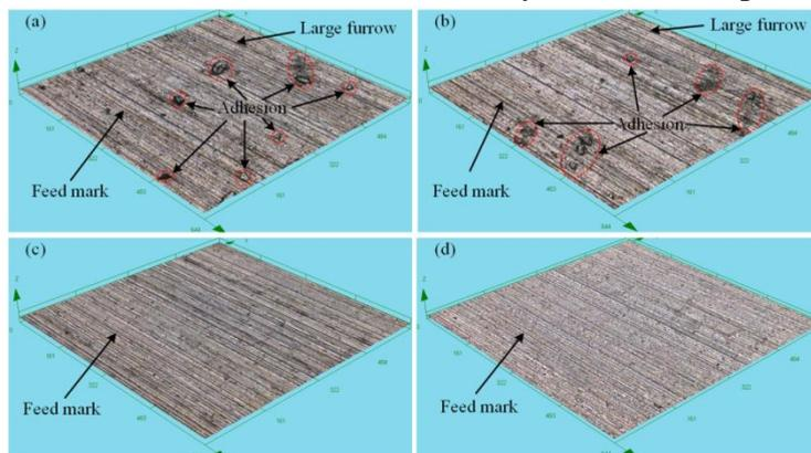
**Fig. 4.** Confocal microscope photos of the machined surface ((a) dry, (b) gas, (c) pure MQL and (d) graphene nanofluid MQL)
