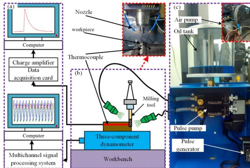
**Fig. 2.** (a) Measurement system, (b) machine tool and (c) MQL system
