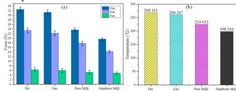
**Fig. 6.** (a) The maximum of milling force and (b) the maximum of milling temperature
