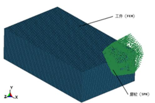
Fig. 7 Simulation model of single abrasive particle wear
