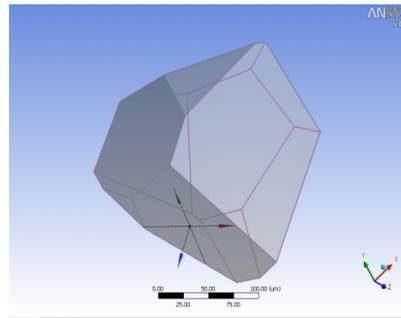
Fig. 5 Irregular abrasive particle after cutting 6 times
