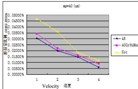
(c) The amount of abrasive loss when ap is 40 $\mu$ m under different velocity and materials
