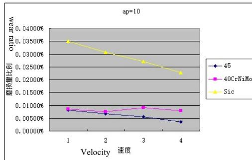
(a) The amount of abrasive loss when  $a_p$  is  $10\mu\text{m}$  under different velocity and materials
