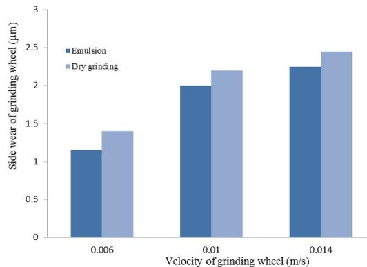
Fig. 11 Results of CBN grinding wheel wear test [13]
