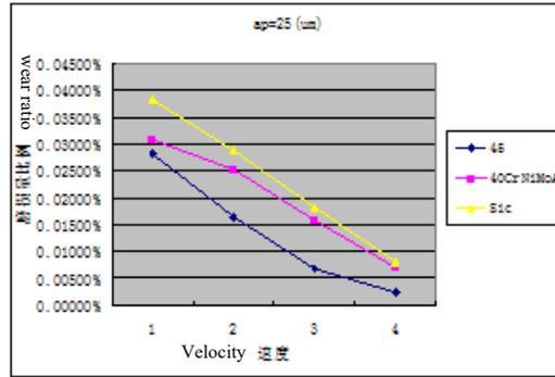
(b) The amount of abrasive loss when ap is 25 $\mu$ m under different velocity and materials
