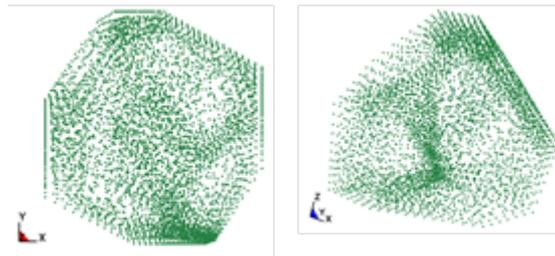
Fig. 6 SPH model of wear abrasive particles
