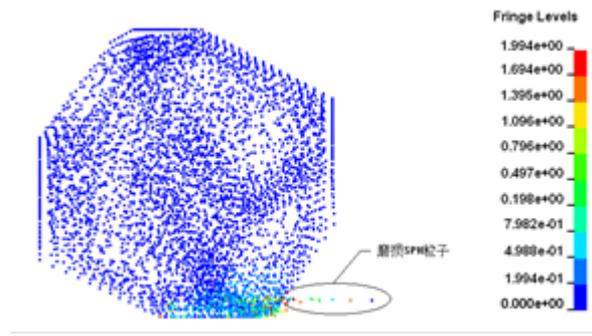
Fig. 8 Worn single abrasive particle
