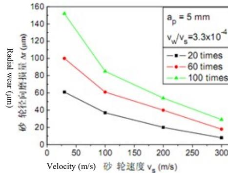
Fig. 10 Relationship between grinding wheel speed and radial wear of grinding wheel [13]
