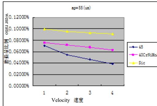
(d) The amount of abrasive loss when ap is 55 $\mu$ m under different velocity and materials
