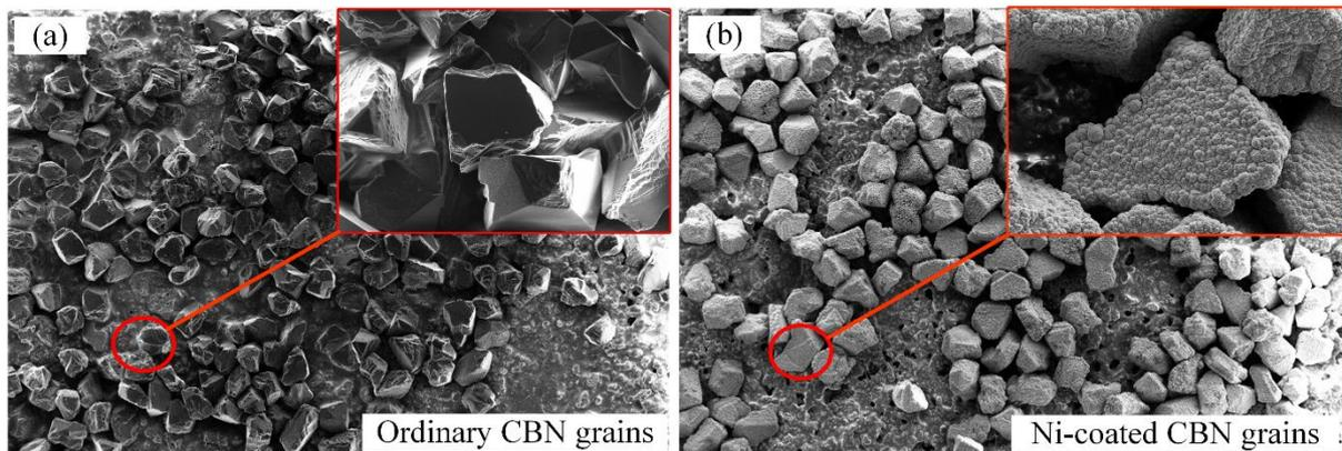
Fig. 1 electron micrograph of ordinary abrasive and coated abrasive
