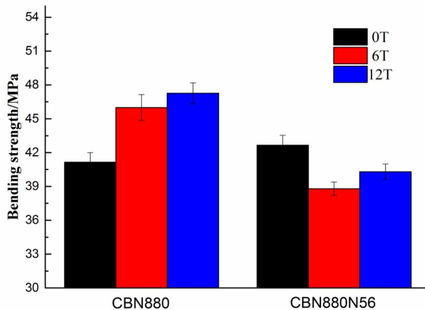
Fig. 3 bending strength of vitrified bond CBN composites with conventional and strong electromagnetic sintering techniques
