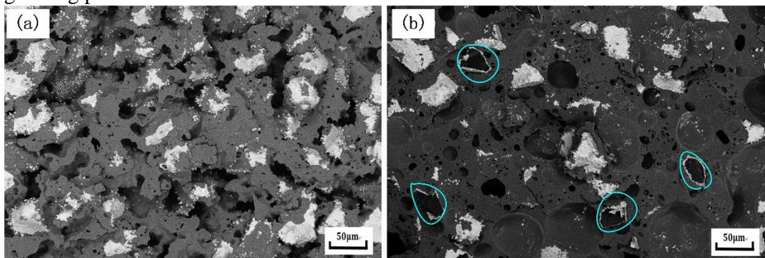
(a) 200× back-reflection image of conventional sintered composites (b) 200× back-reflection image of strong electromagnetic sintered composites
