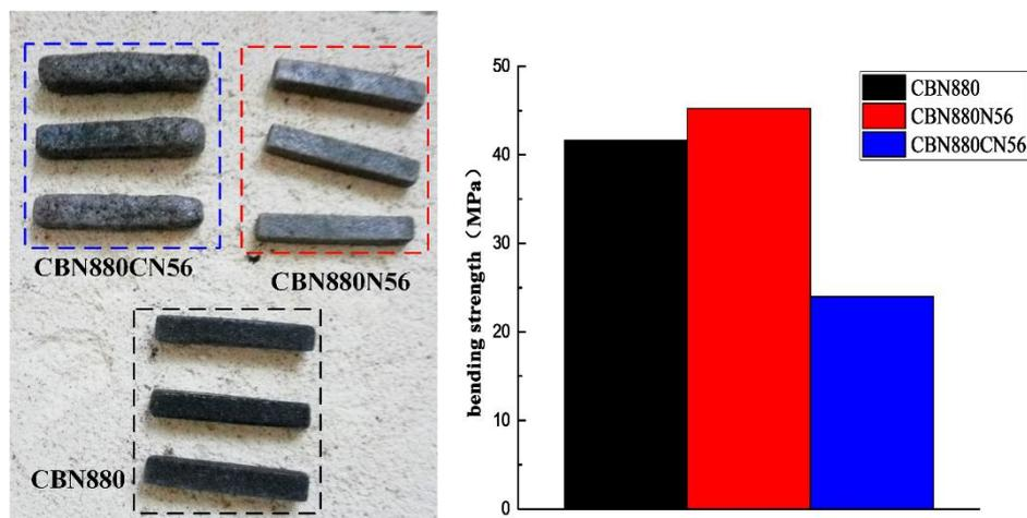
Fig. 2 bending strength of CBN composites specimens
