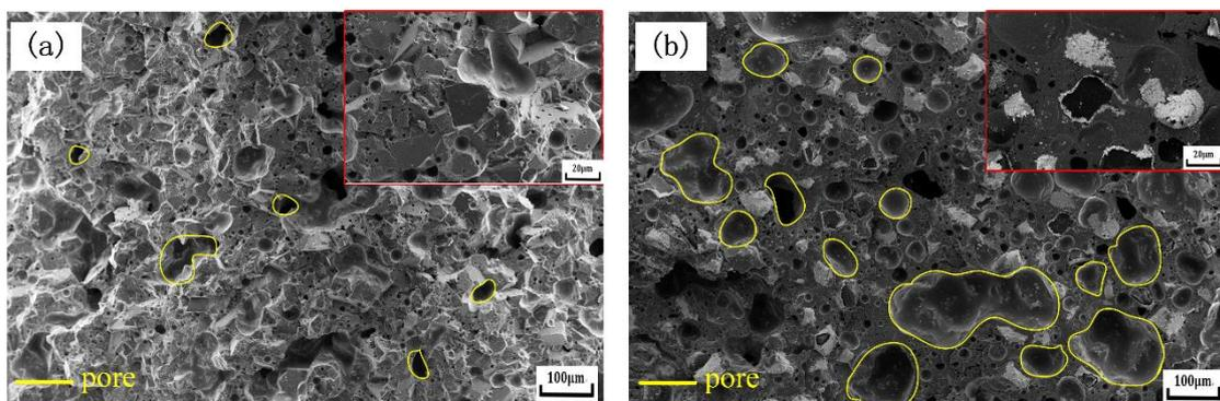
(a) SEM image of CBN composites with ordinary CBN grain, (b) SEM image of CBN composites with Ni-coated CBN grain
