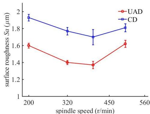
Fig 6: The relationship of surface roughness with the change of spindle speed
