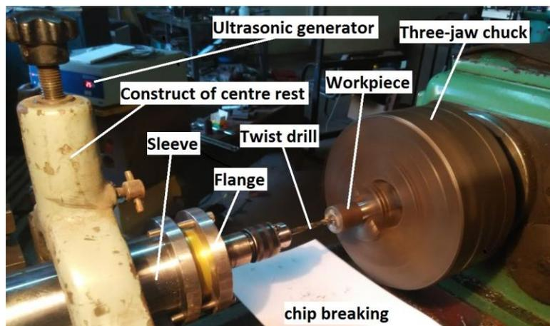
Fig 2: The ultrasonic vibration drilling device
