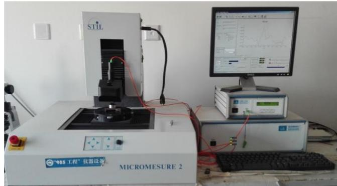
Fig 3: The 3D profiler display system
