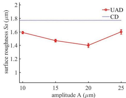
Fig 5: Relationship between surface roughness and ultrasonic amplitude
