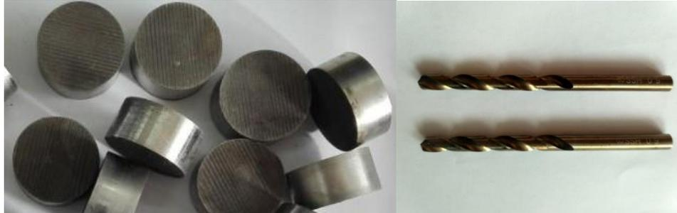
Fig 1: The 45 steel material and drill used in the test
