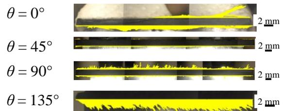
**Fig. 7** Cross section images after cutting tests with a cBN electroplated end-mill for  $f = 0.15$  mm/rev (unidirectional CFRP).
