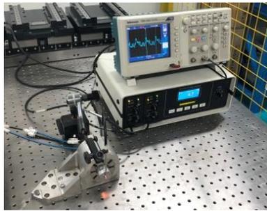
(a) Testing radial motion error
