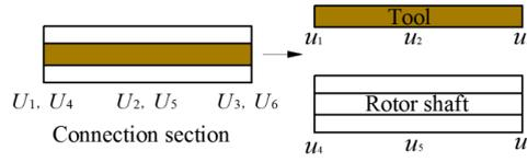
Fig. 6 Model of connection section of rotor shaft and tool
