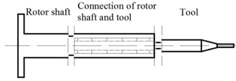
Fig. 4 Schematic diagram of rotor system
