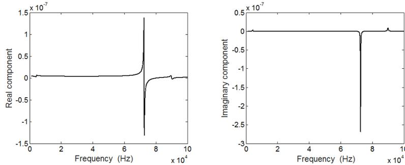
Fig. 7 The first frequency response curve of micro-spindle system
