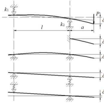
Fig. 3. Deformation schematic diagram of micro-spindle rotor shaft and micro-tool
