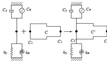
Fig. 5 Model of coupling beam with supporting bearing
