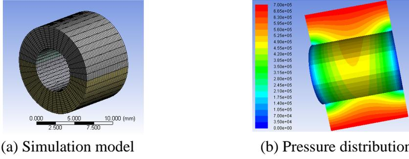
Fig. 2. Simulation of journal porous aerostatic bearing
