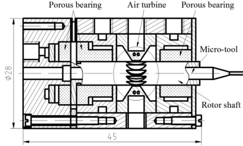
Fig. 1 Structure scheme of the proposed micro-spindle
