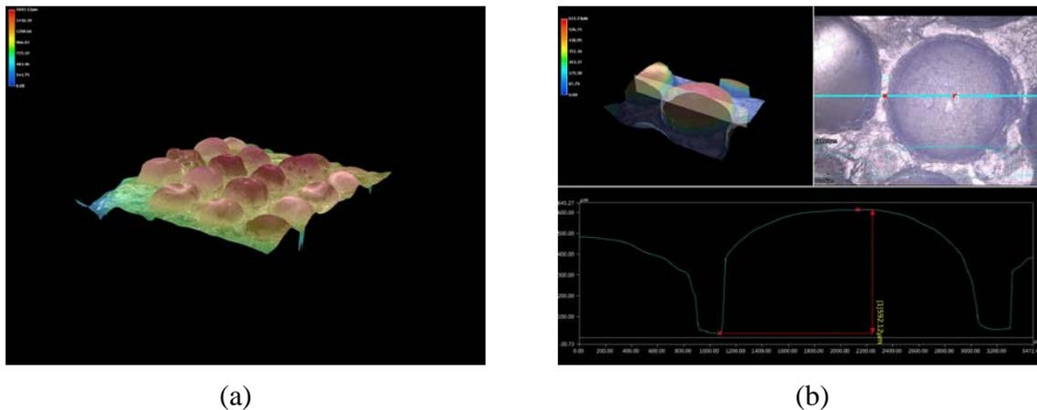
Fig. 3 Morphology of glass surface with columnar array: (a) 3D morphology; (b) profile.
