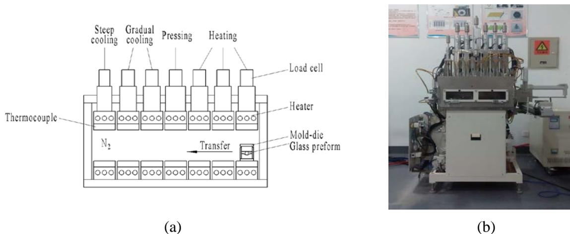
Fig. 2 Glass molding equipment (PF-LF60A): (a) structure diagram; (b) schematic diagram.
