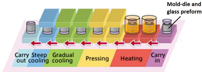
Fig. 1 Process of glass molding process
