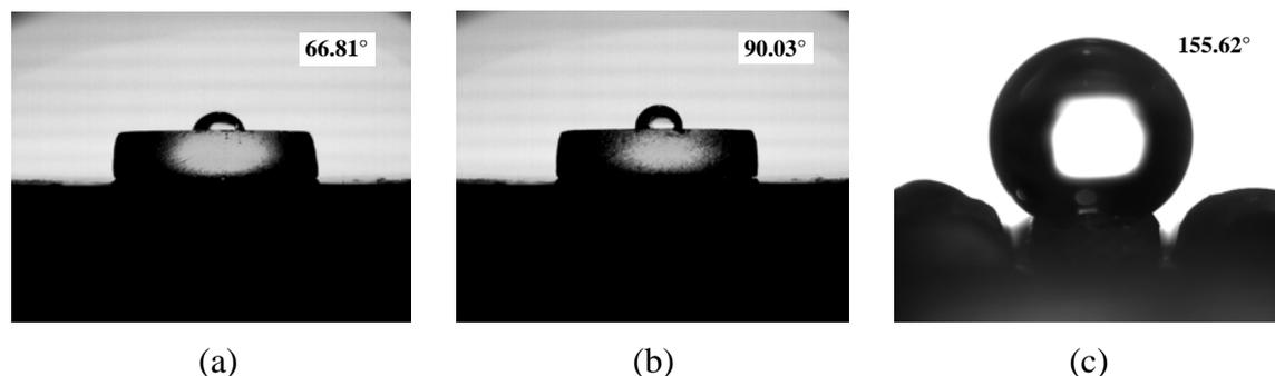
Fig. 4 Contact angles of the glass surface: (a) original glass surface; (b) modified glass surface; (c) glass surface with columnar array after chemical modification.
