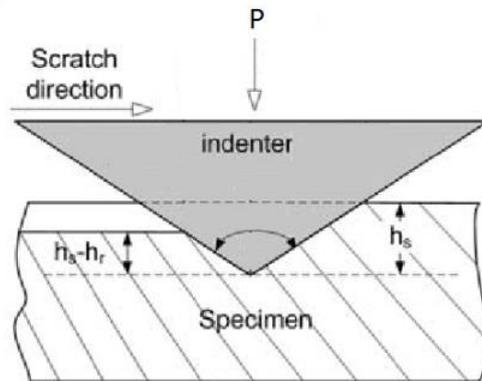
Fig. 1 Illustration of scratch process and elastic rebound
