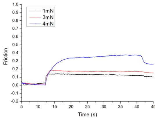
Fig. 6 The friction coefficient curves of various loadings
