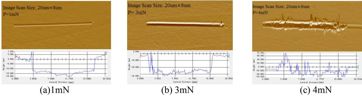
Fig.5 The in-situ scanning morphology and the scratch depth of the constant loading nanoscratch
