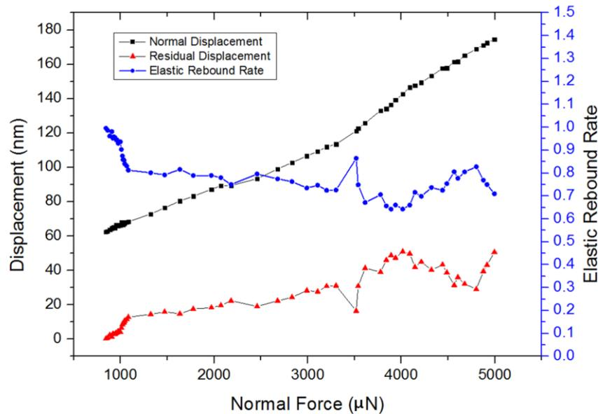
Fig. 9 The curves of the normal displacement, residual displacement and elastic rebound rate
