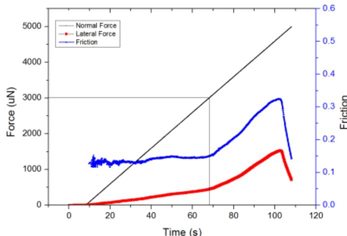
Fig. 4 The relationship of normal force, lateral force and friction during scratch.
