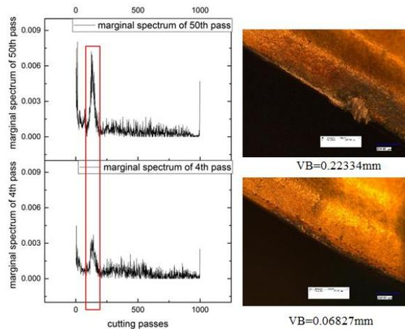
Fig. 4 Comparison of Marginal Spectrum of Spindle Power Signal Obtained from 2nd and 50th Cutting Passes
