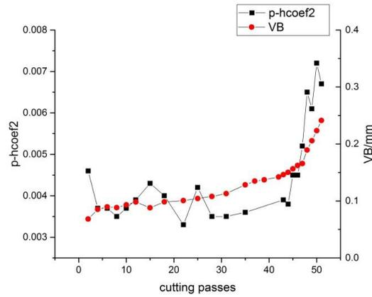
Fig. 5 the Trend of Coefficient p-hcoef2 Obtained with HHT method and Tool Flank Wear
