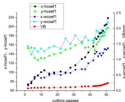
Fig. 2 the Trend of Coefficient x-hcoef1,y-hcoef1 Obtained with HHT method and Coefficient x-wcoef1,y-wcoef1 Obtained with Wavelet Transform method and Tool Flank Wear
