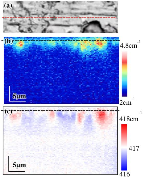
Fig.2 surface image of the surface of BMG (a), and depth profile of the peak-width (b) and peak-shift (c) at 417  $\text{cm}^{-1}$  of the phonon mode .
