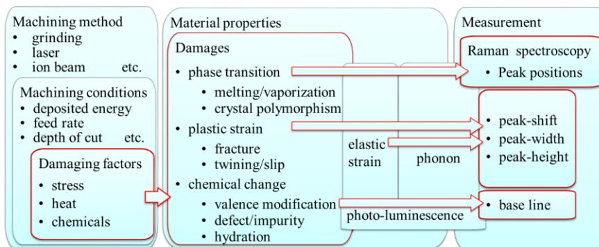
Fig.1 relationship among machining, damaging and measurement of Raman spectroscopy.
