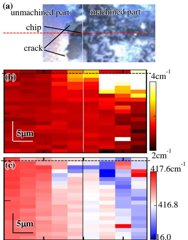
Fig.3 surface image of the surface of NTL (a), and depth profile of the peak-width (b) and peak-shift (c) at 417  $\text{cm}^{-1}$  of the phonon mode .
