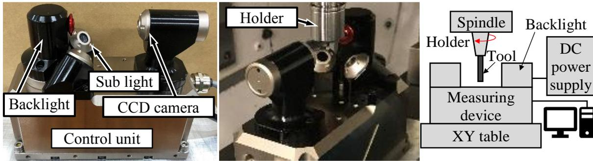
Fig. 2 Overview and schematic illustration of developed tool measuring device.
