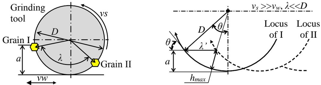
Fig. 1 Schematic illustration of simple grinding model.
