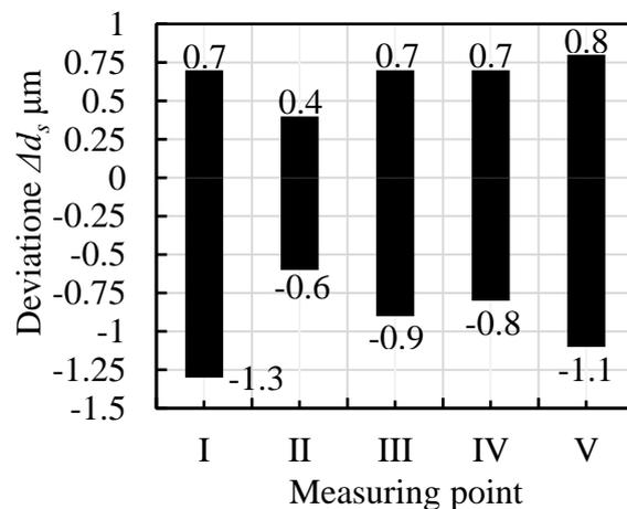
(b) Comparison result of static run-out
