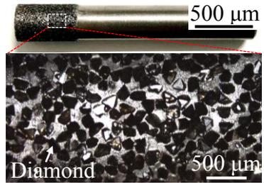
Fig. 4 Diamond electroplated tool (measuring object).
