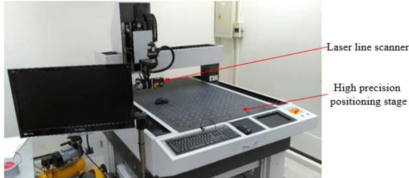
Fig. 1 Picture of the non-contact 3D laser measurement system
