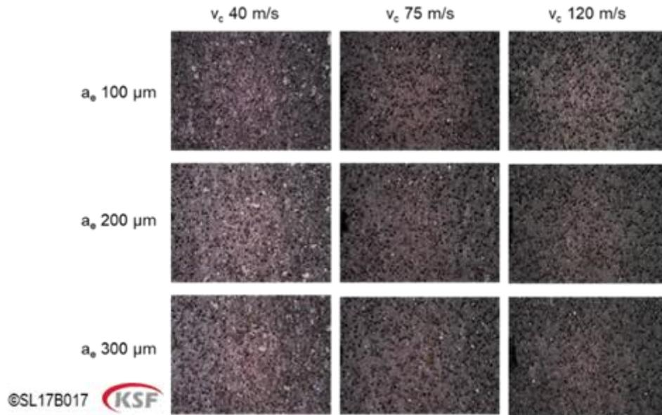
Figure 3. Characteristic Images for each of the grinding tests
