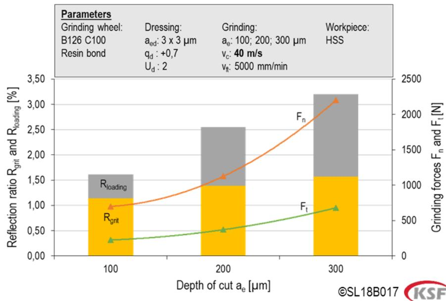
Figure 4. Results for the grinding tests at 40 m/s
