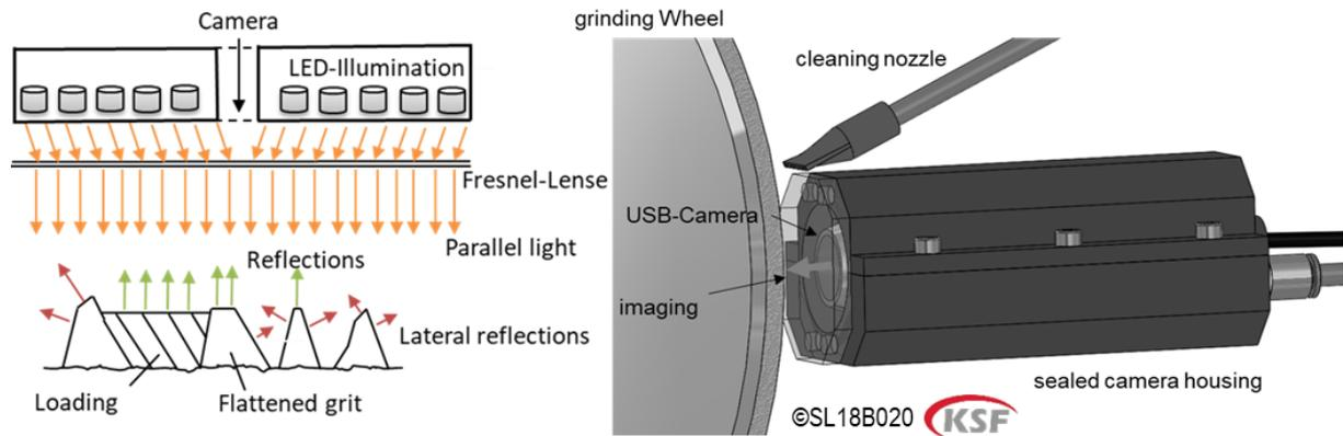
Figure 1. Imaging principle and camera system with housing and cleaning nozzle
