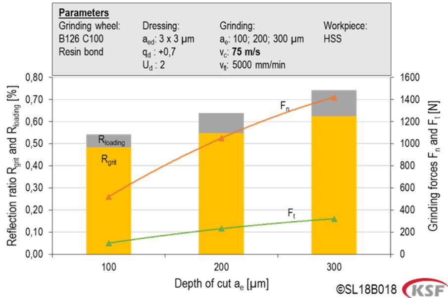
Figure 5. Results for the grinding tests at 75 m/s
