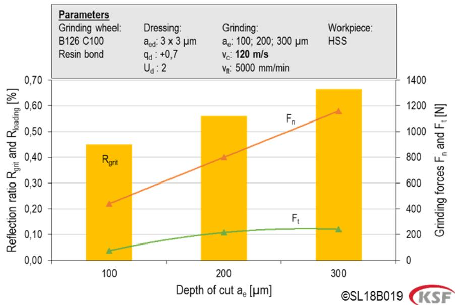
Figure 6. Results for the grinding tests at 120 m/s
