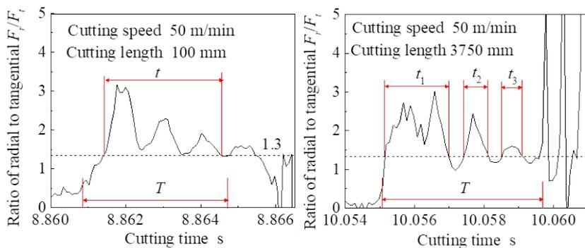
(a) Length of cut: 100 mm (b) Length of cut: 3750 mm
