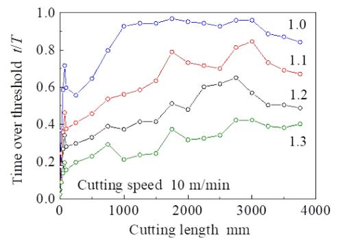
**Fig. 12** Time during width of rake wear land larger than uncut chip thickness in one revolution of spindle (trued up)
