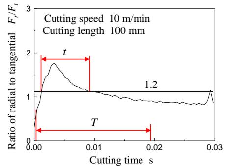
**Fig. 11** Ratio of cutting force in radial direction to cutting force in tangential direction (trued up)
