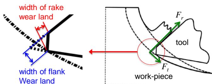
**Fig. 2** Schematic diagram of tool wear in end-milling process
