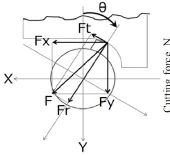
**Fig. 7** Coordinate system of cutting force components in end milling process
