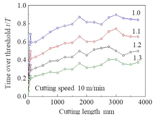
**Fig. 10** Time during width of rake wear land larger than uncut chip thickness in one revolution of spindle (average)
