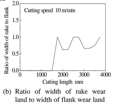
**Fig. 5** Tool wear with progress of end milling (10 m/min)
