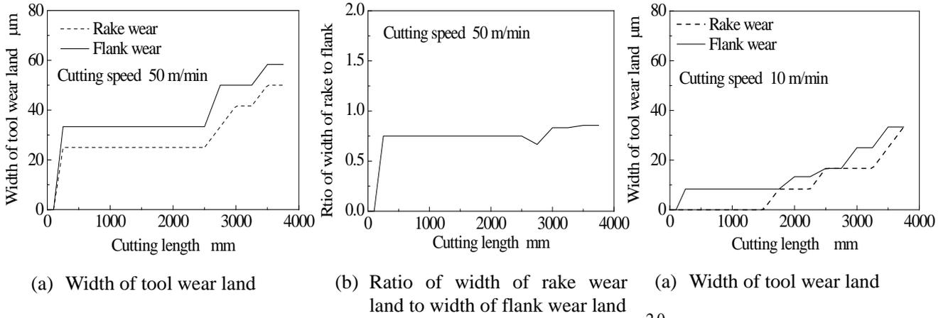
**Fig. 4** Tool wear with progress of end milling (50 m/min)
