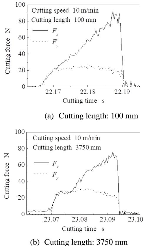
**Fig. 6** Cutting forces in feed direction and normal to feed direction
