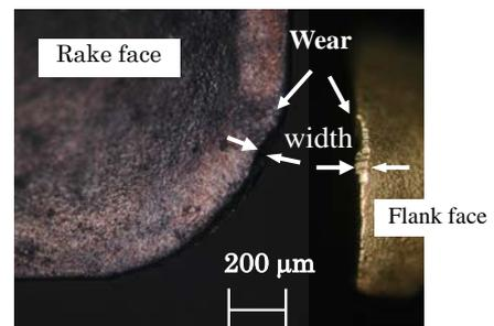
**Fig. 3** Tool wear and its measurement (50 m/min, cutting length: 3750 mm)
