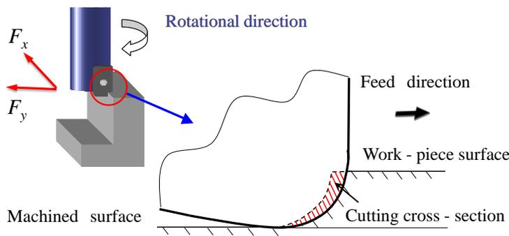
**Fig. 1** Schematic diagram of end milling process
