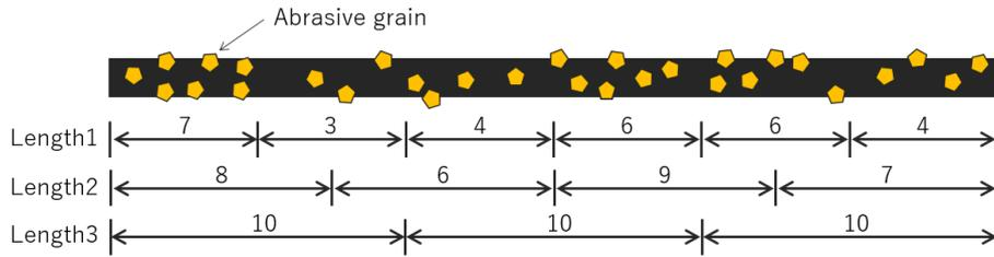
Fig.4 Statistical evaluation of the wire surface topography
