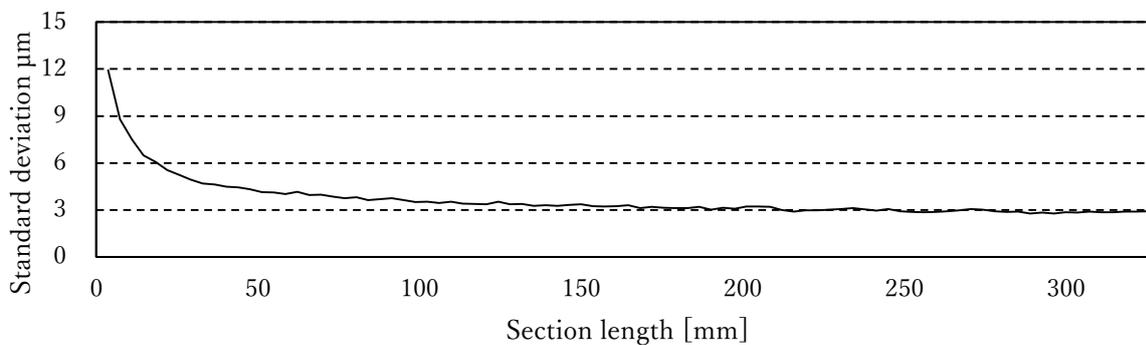
Fig.9 Standard deviation of the distance between nearest abrasive grains per section length
