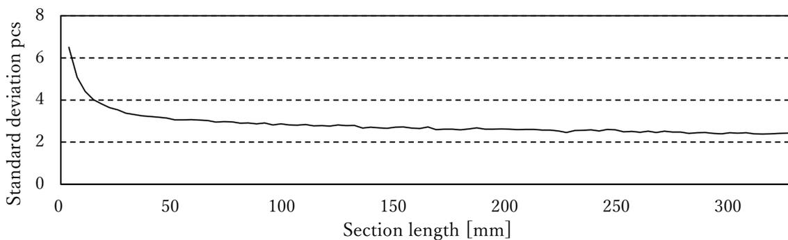
Fig.8 Standard deviation of the number of abrasive grain per section length
