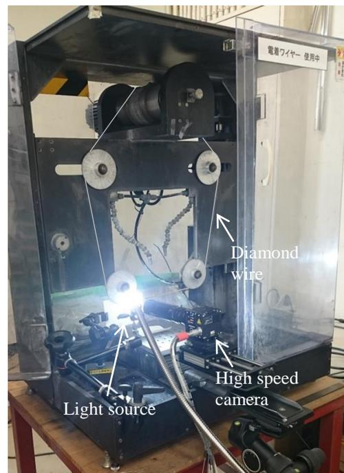
Fig.1 Diamond wire saw
