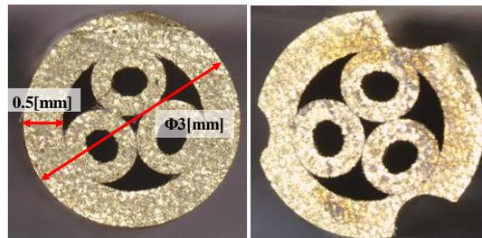
Fig. 3 Cross section photographs of electrodes
