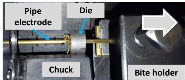
Fig. 2 Method of cutting method using the die
