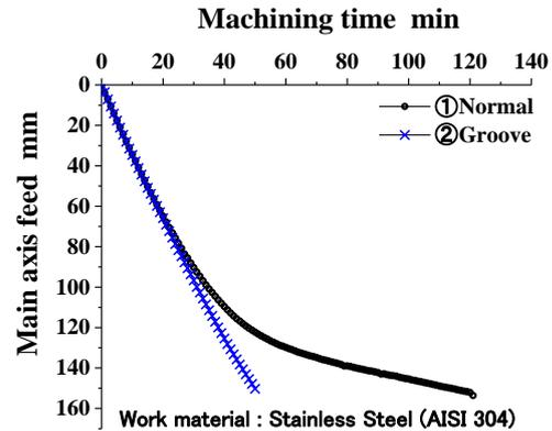
Fig. 5 Transition of the main axis with respect to the machining time (Stainless Steel)
