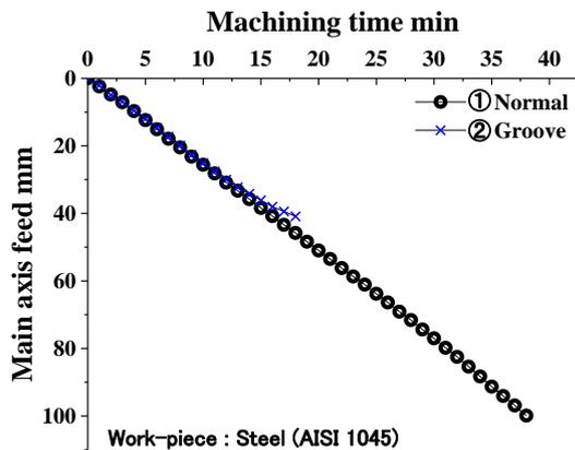
Fig. 4 Transition of the main axis with respect to the machining time (Steel)
