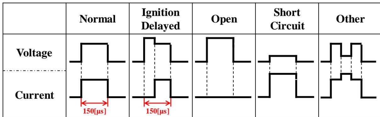
Fig. 6 Classification of discharge waveforms
