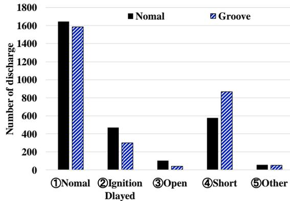
Fig. 7 Classification of discharge state at 70 mm machining depth
