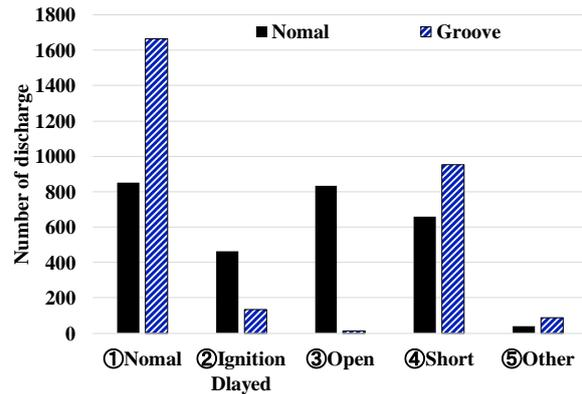
Fig. 8 Classification of discharge state at 120 mm machining depth
