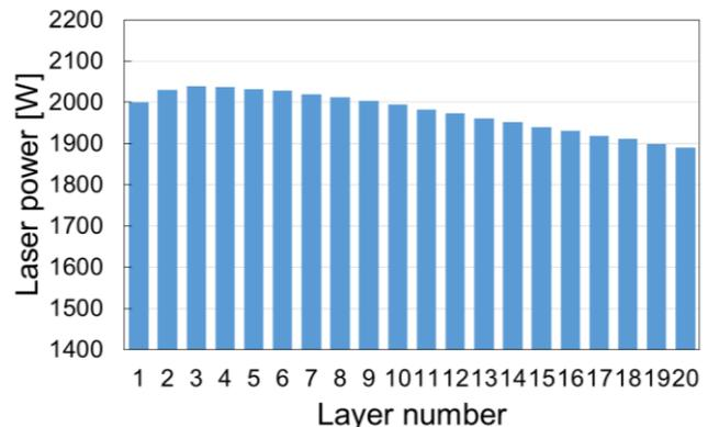
Fig. 4 Generated Laser command for each layer
