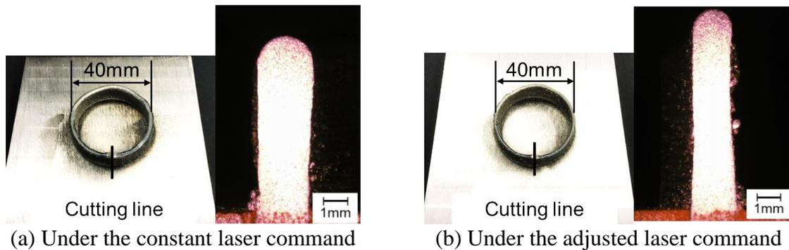
Fig. 12 Cylinder deposited objects and cross sections
