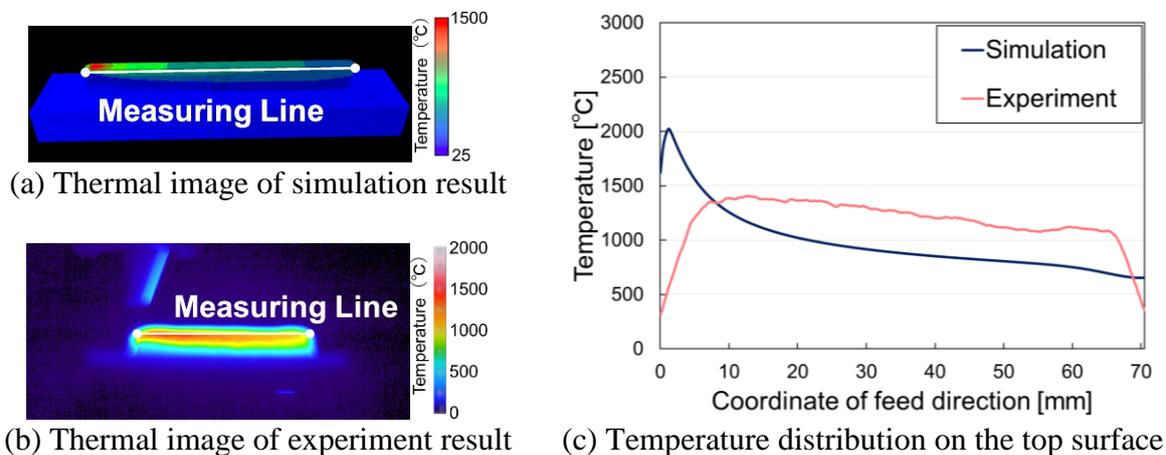
Fig. 7 Thermal image and temperature distribution after the 20th layer deposition
