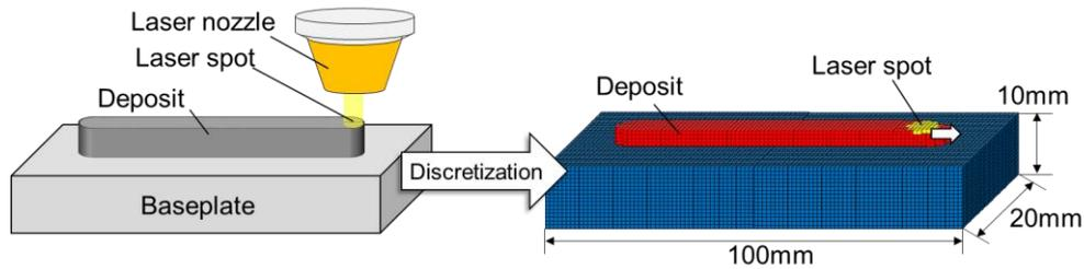
Fig. 2 Three-dimensional heat conduction simulation model
