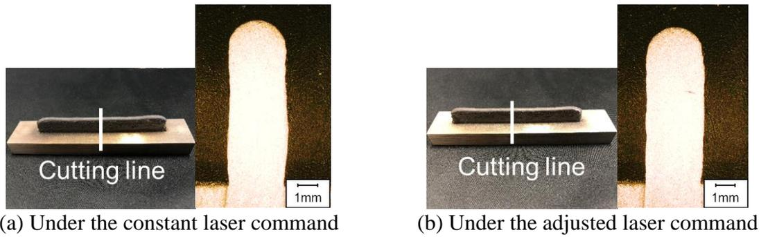
Fig. 11 70-mm long thin wall deposited objects and cross sections
