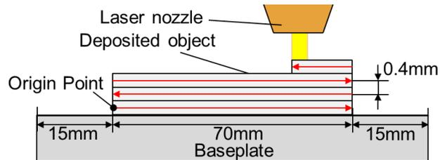
Fig. 6 Deposition trajectory for thin-wall deposited object
