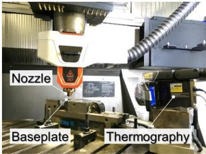
Fig. 5 Experimental setup
