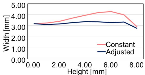
Fig. 10 Relation between width and height of thin wall deposited objects
