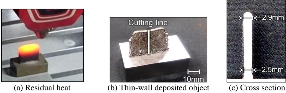
Fig. 1 Deformation due to overheating in directed energy deposition
