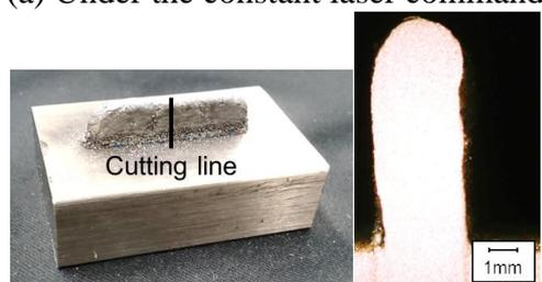
Fig. 9 30-mm long thin wall deposited objects and cross sections
