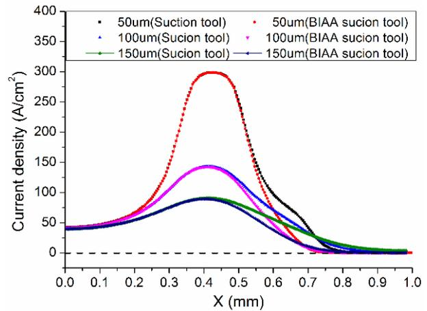
Fig. 4 Current density distribution in ECM with suction tool under different IEG
