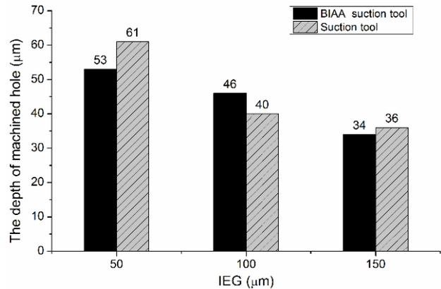
Fig. 7 The depth of machined hole under different IEG
