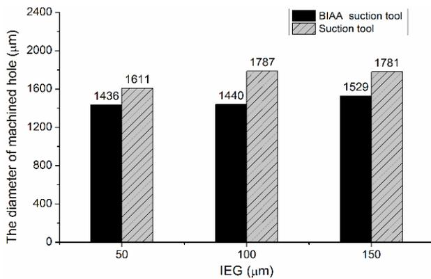
Fig. 6 Diameter of machined hole under different IEG
