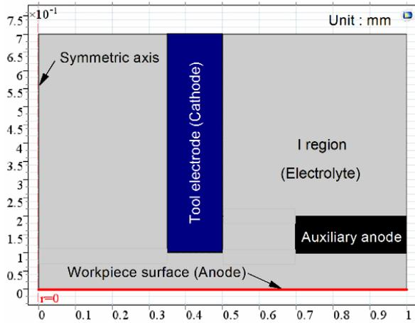
Fig. 3 Two-dimensional symmetric electric field analysis model
