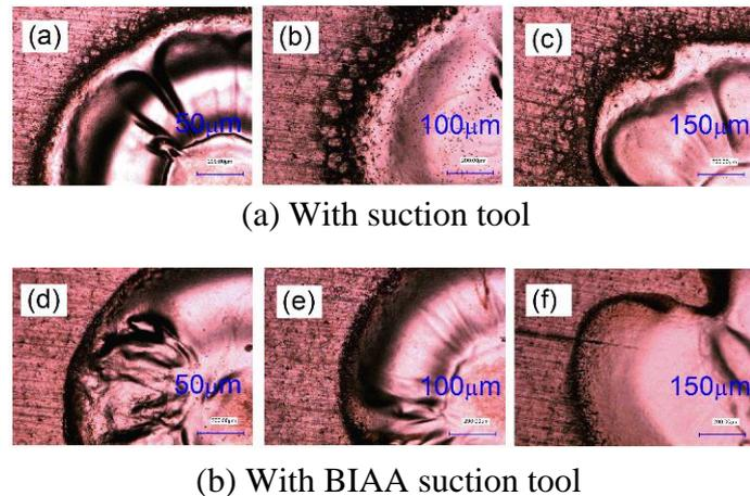
Fig. 8 Stray corrosion on the edge of the machined hole
