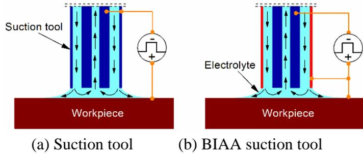
Fig.1 Structure and principles of suction tools
