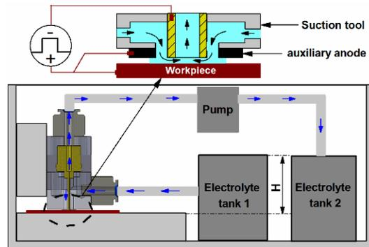
Fig. 2 Schematic of ECM with BIAA suction tool test equipment
