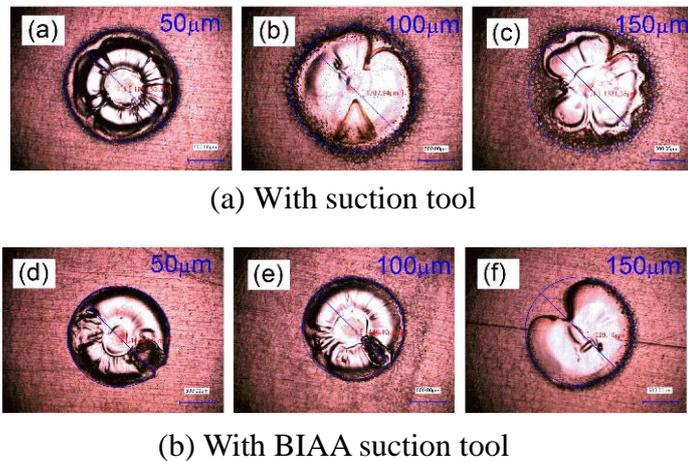
Fig. 5 The machined hole by ECM under different IEG
