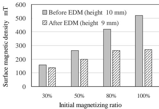
Fig. 4 Difference between the magnetic flux density before and after machining in different initial magnetizing ratio
