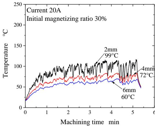
Fig. 6 The magnet internal temperature of each height in initial magnetizing ratio of 30% during machining under rough machining condition
