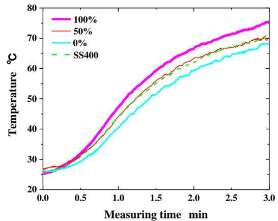
Fig. 7 Change in temperature rise in each initial magnetizing ratio and SS400
