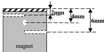
Fig. 3 Measurement position of internal temperature at simultaneous measurement
