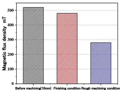
Fig. 1 Difference between the magnetic flux density before and after machining
