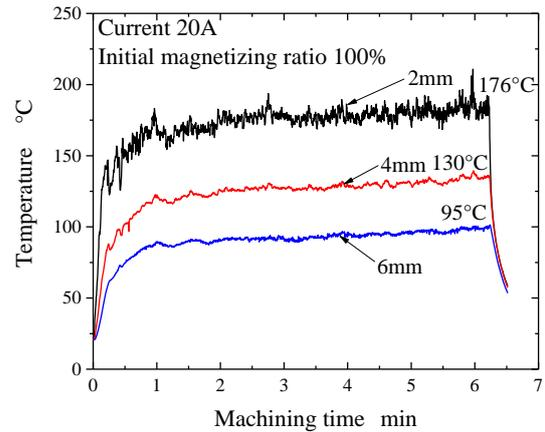
Fig. 5 The magnet internal temperature of each height in initial magnetizing ratio of 100% during machining under rough machining condition
