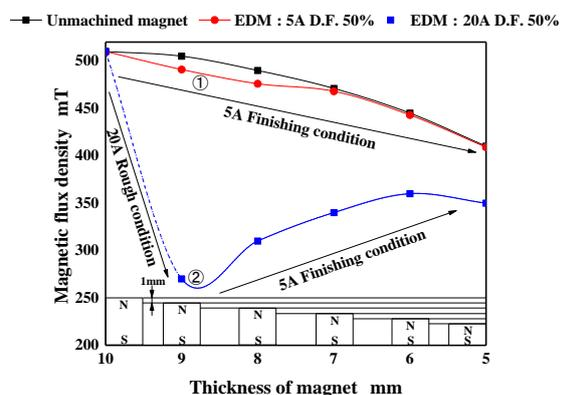
Fig. 2 Change in the magnetic flux density in each magnet height due to the difference of the discharge condition
