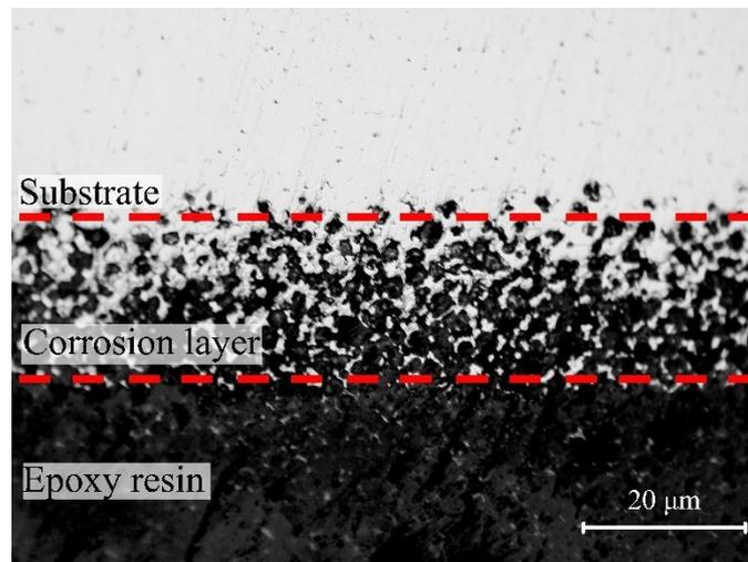
Fig. 4 The cross section photo of the corrosion layer formed in the  $\text{Na}_2\text{CO}_3$  solution
