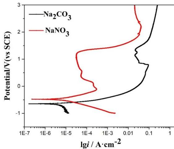
Fig. 2 Potentiodynamic polarization curves of the tungsten alloy
