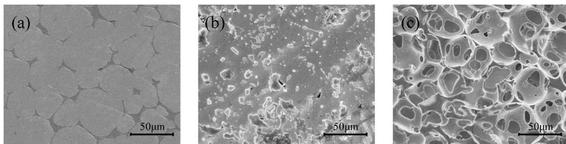
(a) Initial surface (b) Treated in the  $\text{NaNO}_3$  solution (c) Treated in the  $\text{Na}_2\text{CO}_3$  solution
