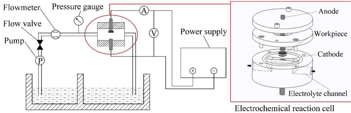
Fig. 1 Anodic treatment experimental system
