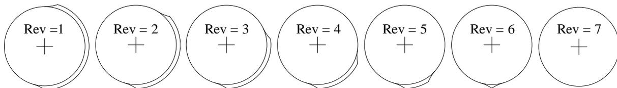
Figure 4: Effect of non-integer speed ratio on workpiece surface pattern
