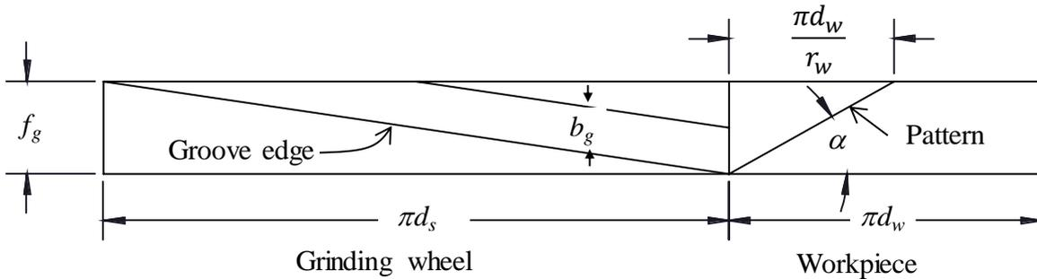
Figure 3: Groove Geometry
