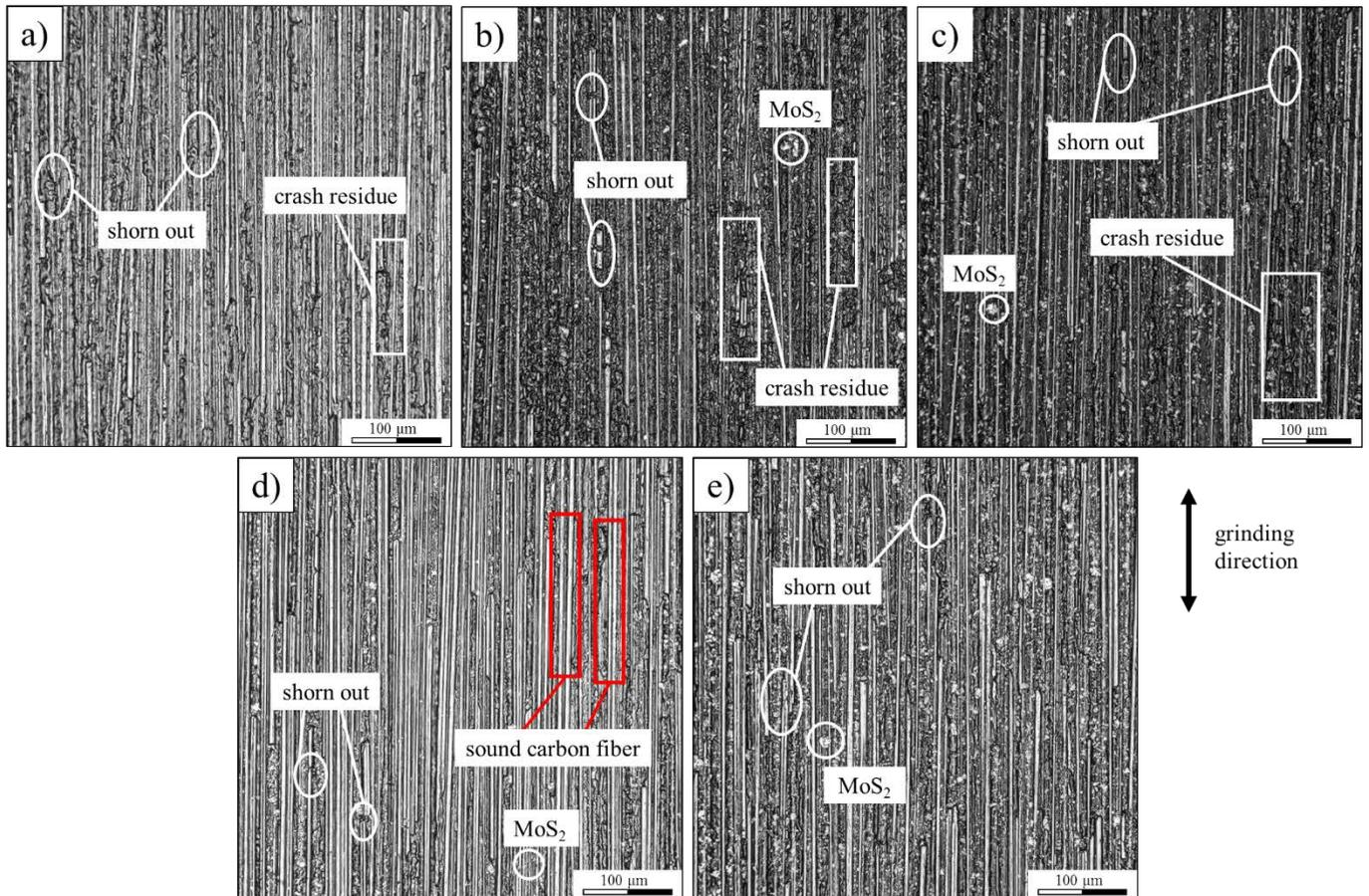
Fig. 4 Schematic of the surface morphology of ground CFRPs with concentration of a) 0% b) 3% c) 6% d) 9% e) 12% nano MoS<sub>2</sub> MQL grinding
