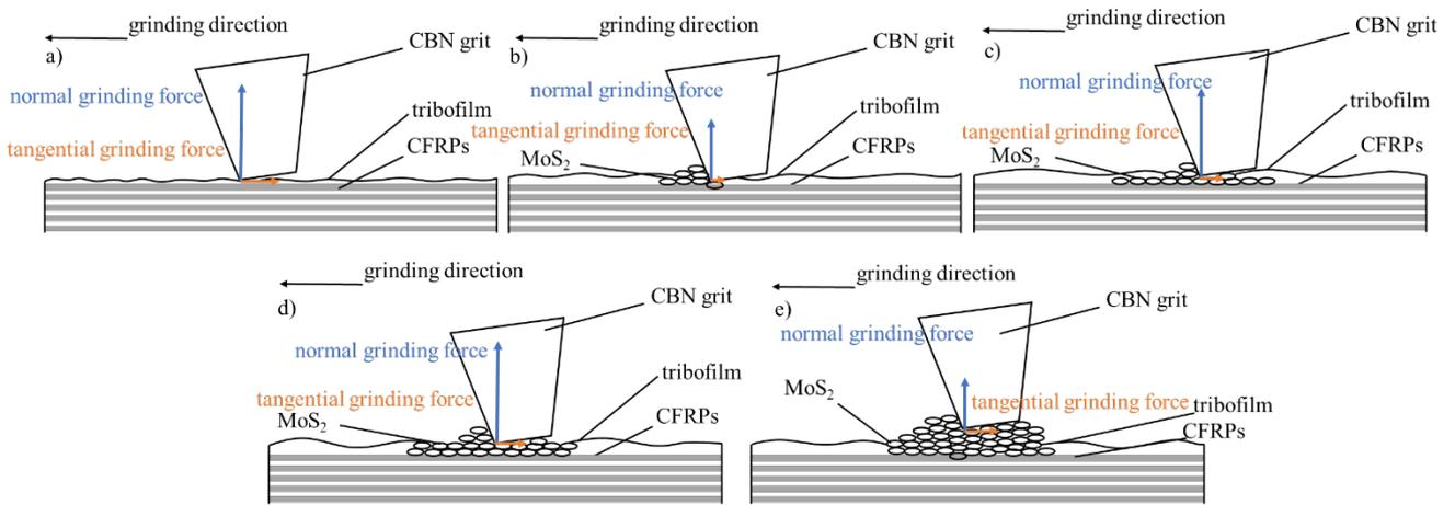
Fig. 5 Schematic of CFRPs grinding with a) 0% b) 3% c) 6% d) 9% e) 12% nano MoS<sub>2</sub> concentrations MQL grinding
