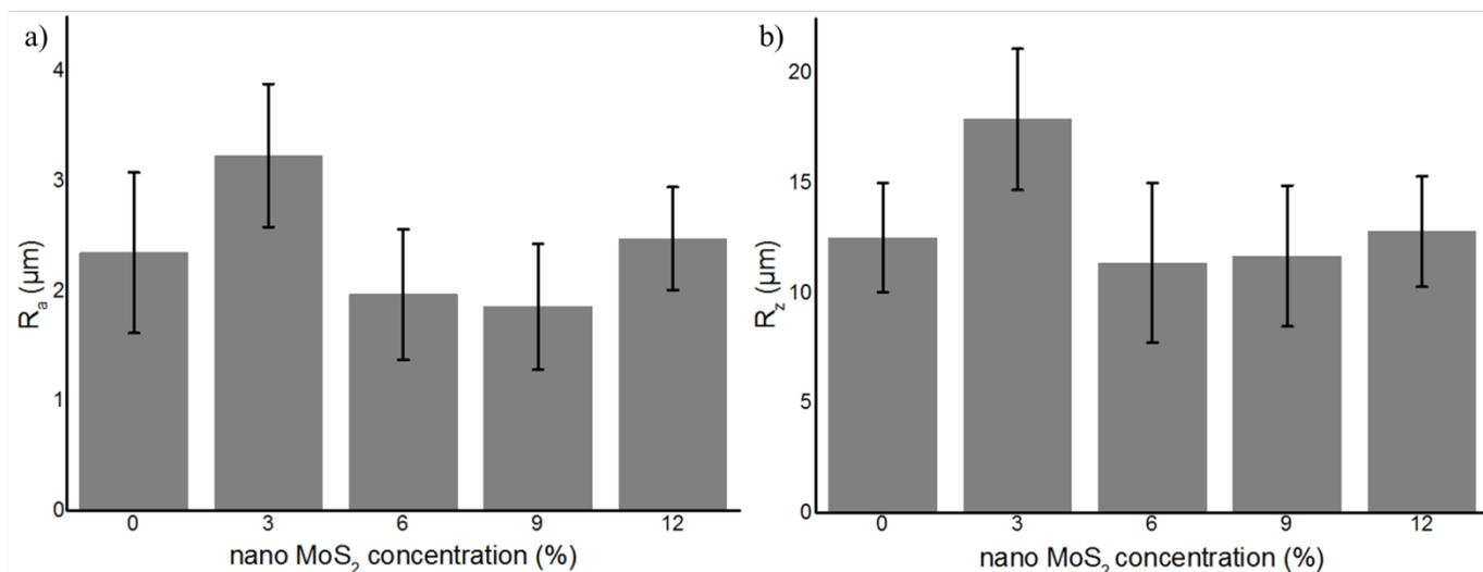
Fig. 3 Schematic of surface roughness under various nano MoS<sub>2</sub> concentrations in MQL grinding a)  $R_a$  b)  $R_z$
