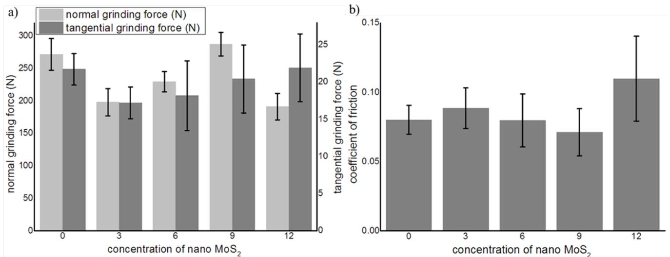
Fig. 2 Schematic of a) average normal grinding force and average tangential grinding force and b) coefficient of friction
