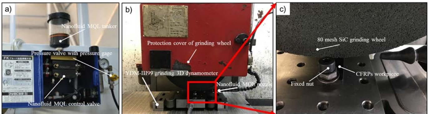
Fig. 1 a) nanofluid MQL transfer system; b) grinding operation setup; c) local magnification of grinding area
