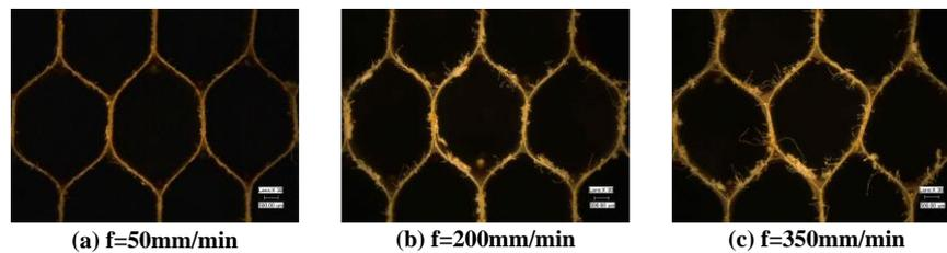
Fig.9 Surface morphology of different feed rate
