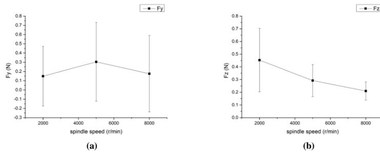
Fig.13 Influence of spindle speed on grinding force
