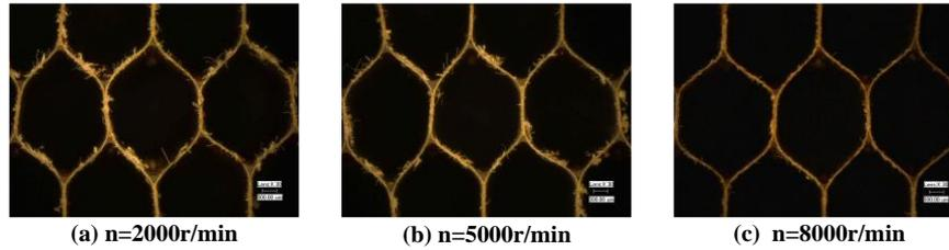
Fig.7 Surface morphology of different cutting speed
