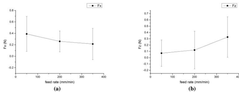
Fig.14 Influence of feed rate on grinding force
