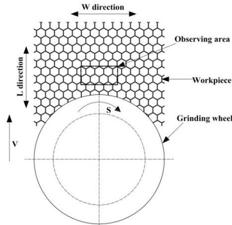
Fig.4 Diagram of grinding process
