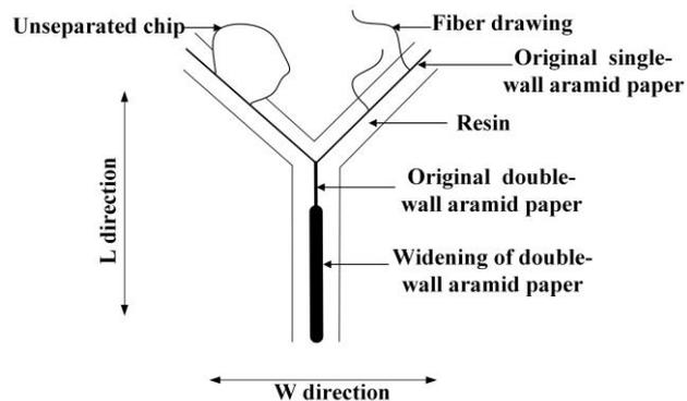
Fig. 6 Diagram of processing defects
