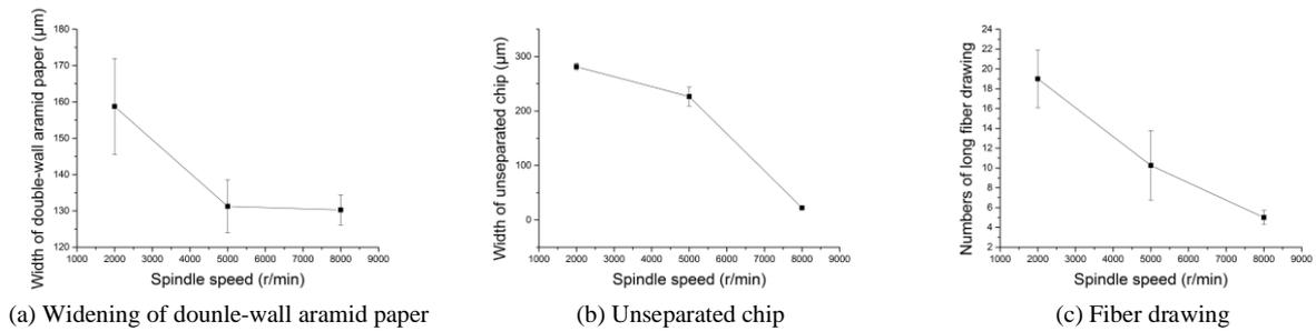
Fig.8 Influence of spindle speed on three kinds of processing defect
