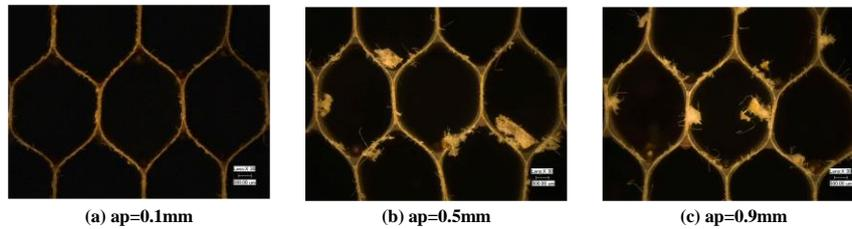
Fig.11 Surface morphology of different cutting depth
