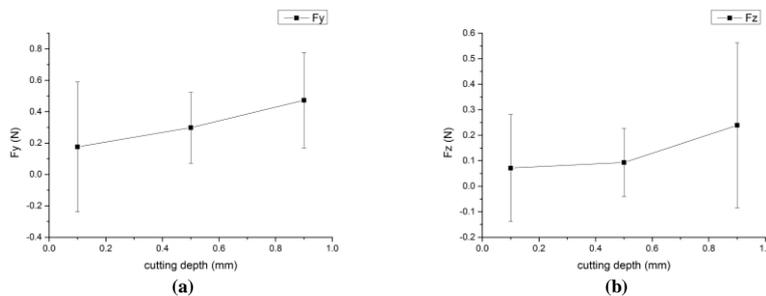
Fig.15 Influence of cutting depth on grinding force
