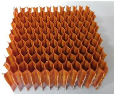
Fig.1 A sample of high-density Nomex honeycomb core
