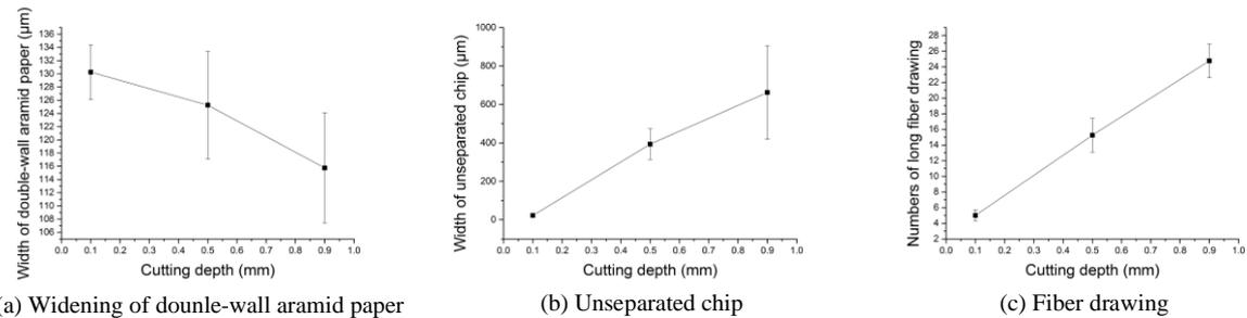
Fig.12 Influence of cutting depth on three kinds of processing defect
