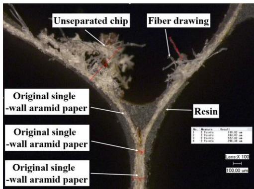
Fig. 5 Physical picture of processing defects
