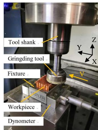
Fig.2 Structure diagram of cup-type diamond wheel Fig.3 Overview of experimental setup
