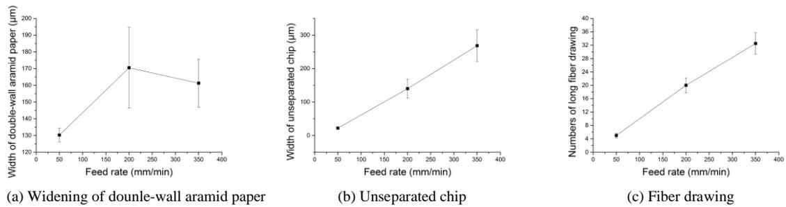
Fig.10 Influence of feed rate on three kinds of processing defect
